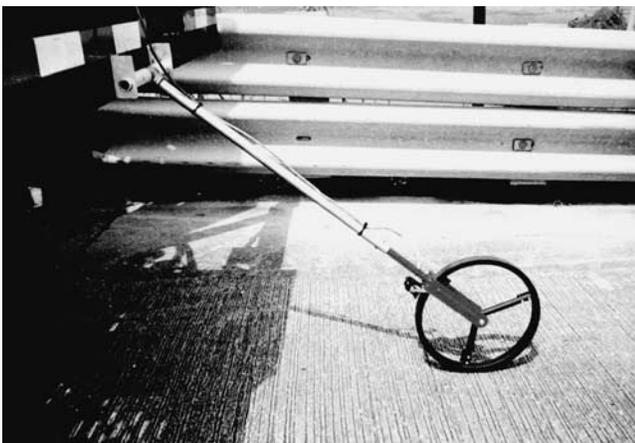
Figure A13. Surveyor's wheel attached to back of truck.
