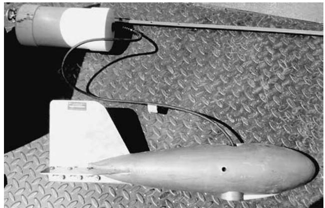
*Figure B34. Close up of sounding weight showing wedge on leading edge of sonar.*
