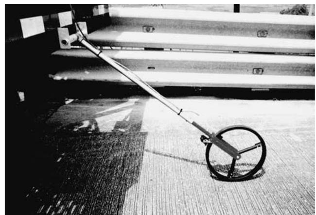
Figure 26. Surveyors wheel mounted to rear bumper of truck.
