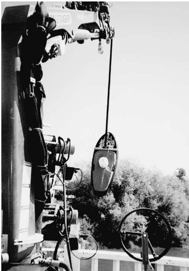
Figure A18. Kneeboard with wireless sonar (note PVC instrument enclosure where transducer and radio modem are located).
