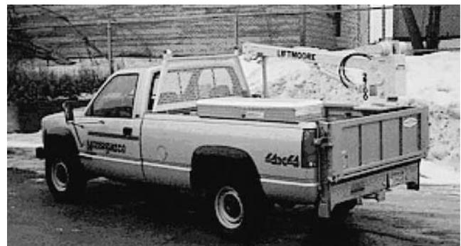
Figure 10. Application of winch concept on a non-articulated crane.
