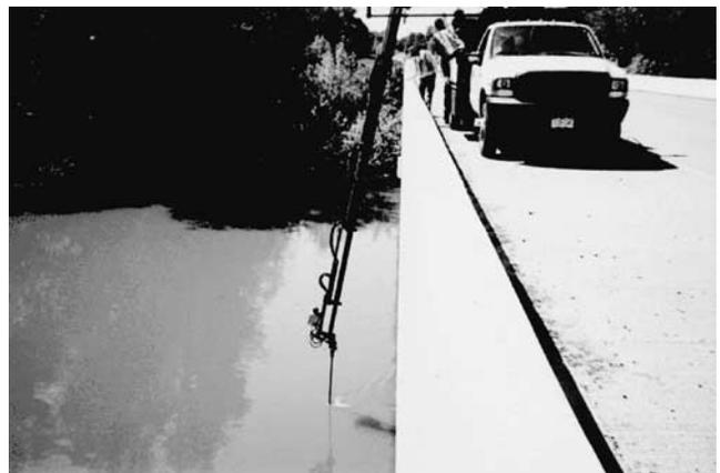
Figure B30. Sonar in the water as the truck is moving across the bridge during a cross section measurement.
