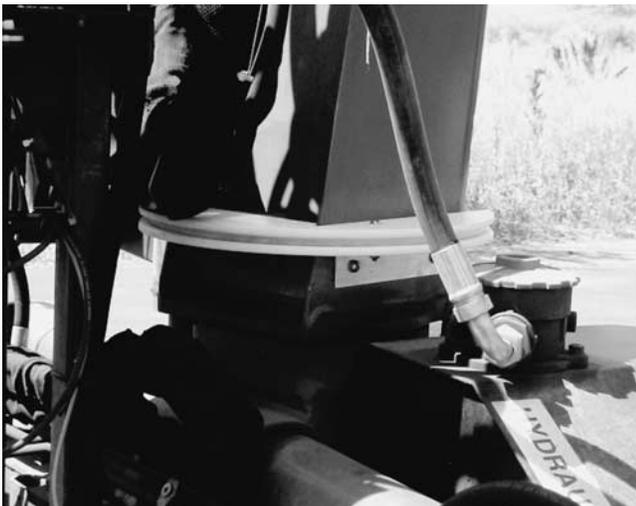
Figure 22. Attachment for crane azimuth measurement using draw wire.
