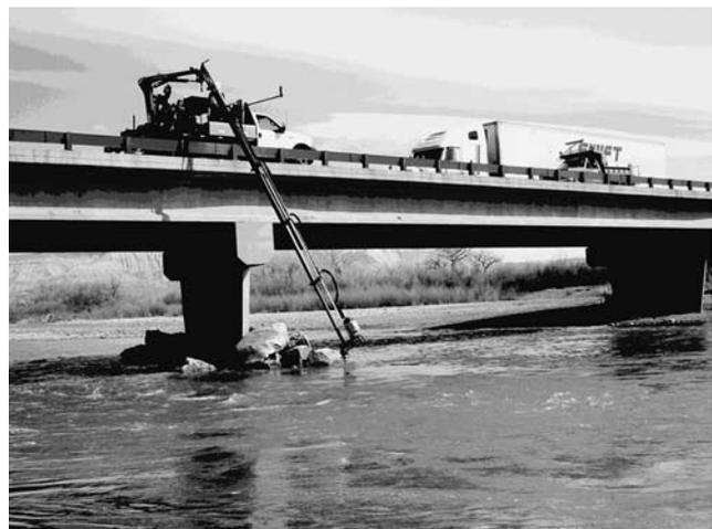
Figure A1. Articulated arm truck making a scour measurement.
