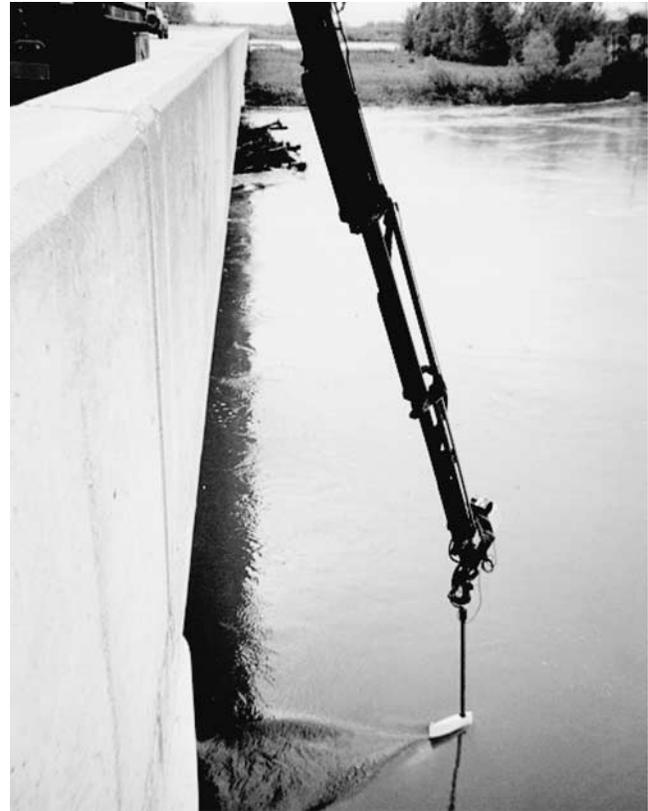
Figure 29. Modified streamlined probe with swivel capability and longer extension.
