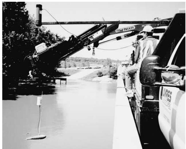
Figure 32. Sounding weight with wireless sonar.
