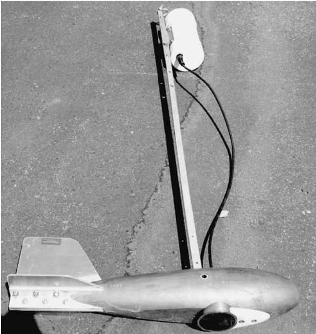
Figure 33. Sonar mounted in bottom of sounding weight with shim to transition flow off the nose.
