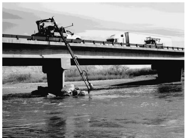
Figure 43. Using the crane to sweep arcs on downstream side of Colorado River bridge.
