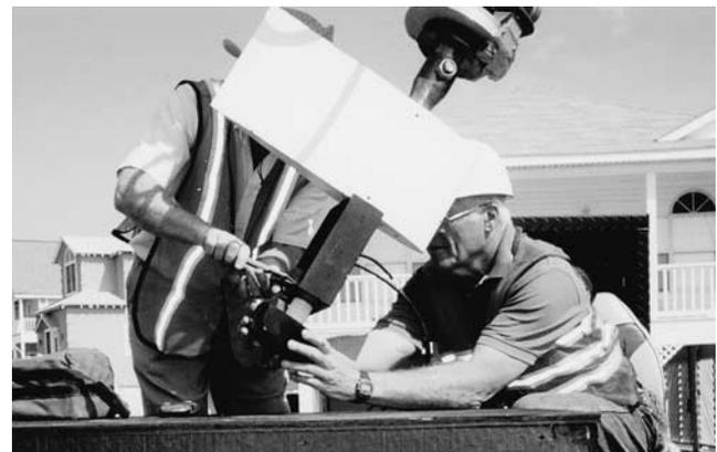
Figure 14. Mounting the Twinscope™ transducer for field testing.
