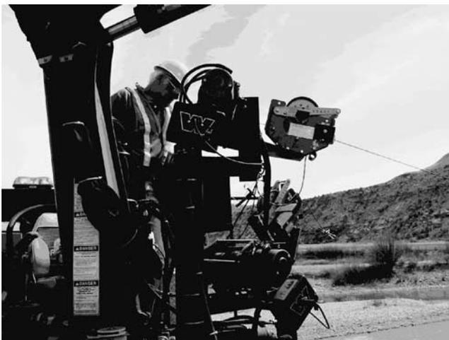
Figure B6. Using a single winch to position sounding weight with Marsh-McBirney.
