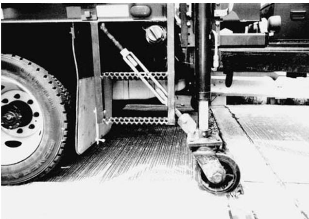
Figure 34. Turnbuckle to stabilize the hydraulic jacks for the crane.
