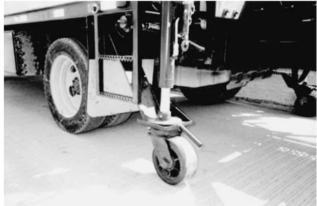
Figure 35. Final design for castor system.
