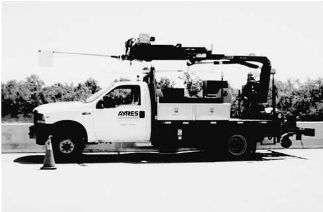
Figure A4. PK4501C crane mounted on the back of a F450 truck.
