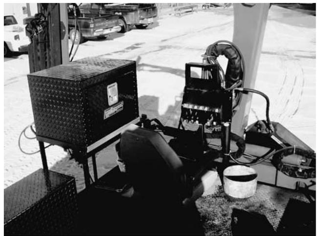
Figure 21. Instrument shelter for computer and relocated hydraulic controls.
