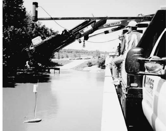
Figure A23. Wireless sonar in a sounding weight.
