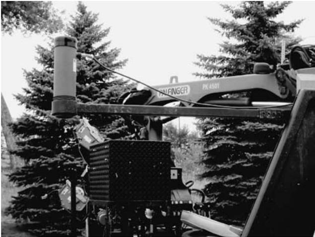
Figure 25. Acoustic stage sensor used to measure distance to the water surface.
