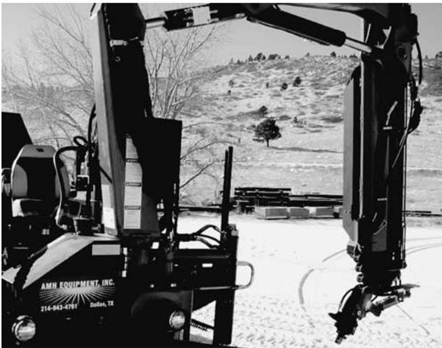
Figure 19. Rotator after modifications to provide tilt capability.
