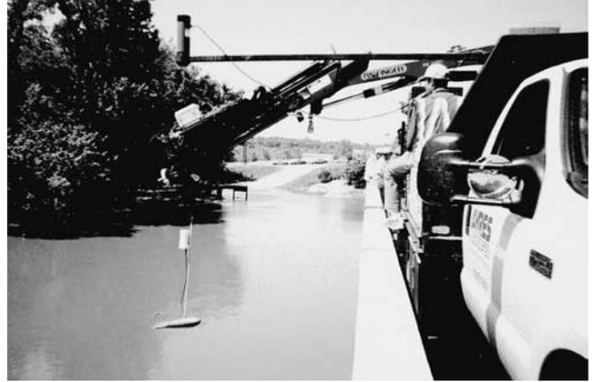
Figure 53. Sounding weight with a wireless sonar being tested in Indiana.
