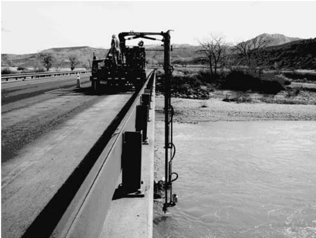
Figure B1. Crane on downstream side of bridge near scour hole.
