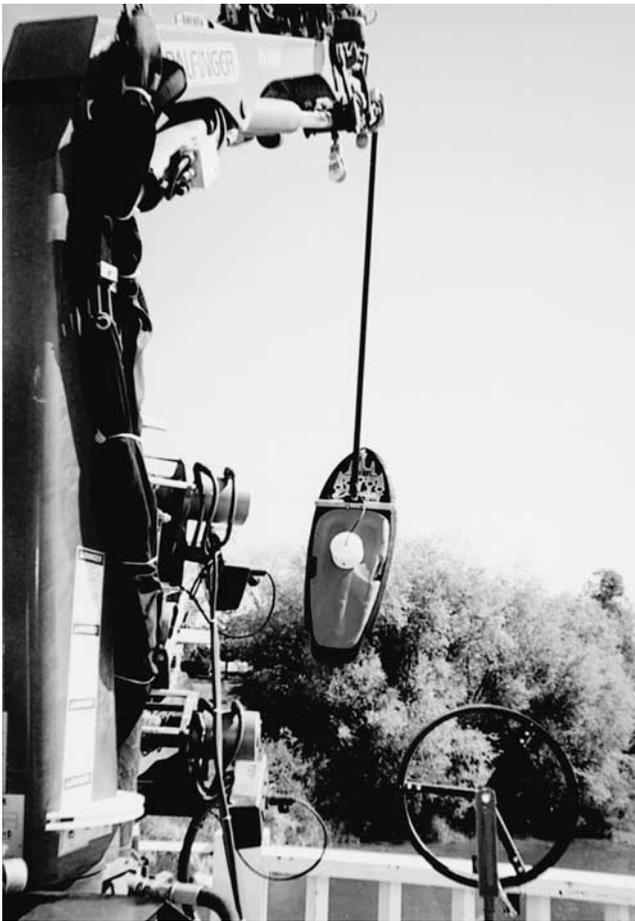
Figure 30. Kneeboard with wireless sonar being deployed with a rigid frame.
