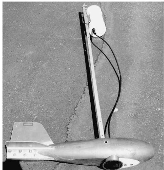
Figure A24. Shim on bottom of sounding weight.
