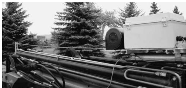
Figure 24. Draw wire used to measure linear extension of crane.
