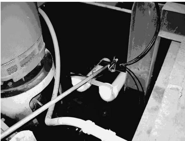
Figure 12. Pontoon float with transducer adjacent to pump intake in the CSU Hydraulics Laboratory.
