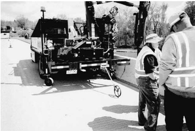
Figure B17. Cross section measurement with castors deployed and survey wheel in place to measure distance traveled.
