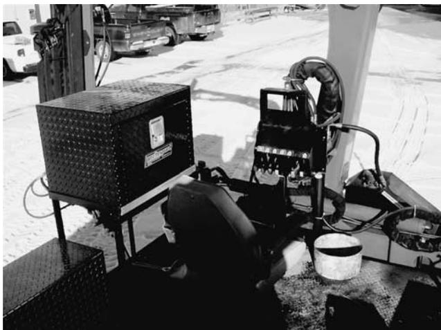
Figure A9. Instrument shelter for computer and relocated hydraulic controls.
