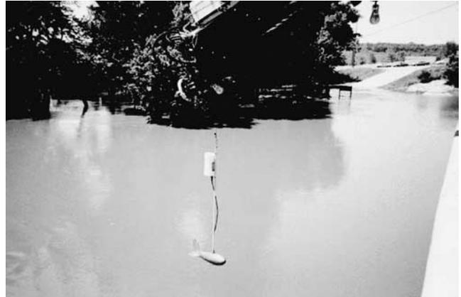
*Figure B33. Sounding weight with sonar.*
