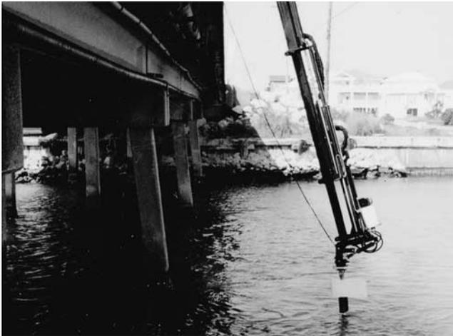
Figure 15. Positioning the Twinscope™ transducer upstream of a pile.
