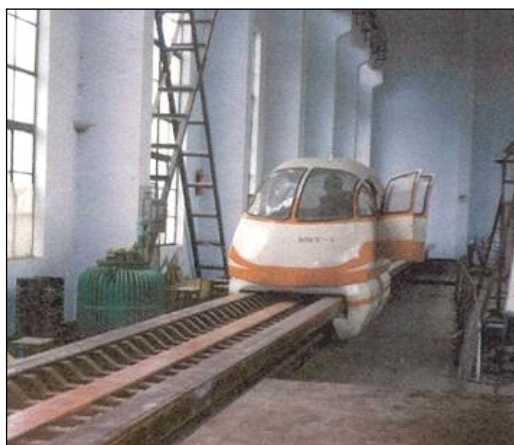
FIGURE 6 Low-speed maglev train developed by Southwest Jiaotong University.
