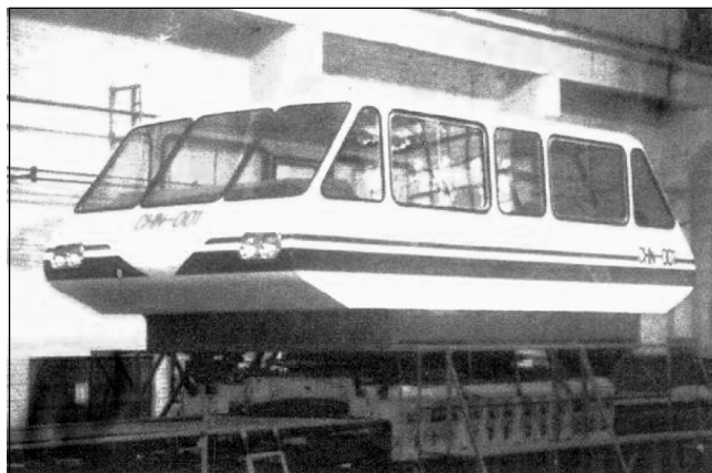
FIGURE 5 Six-ton, single-bogie truck maglev train developed primarily by Railway Academy.
