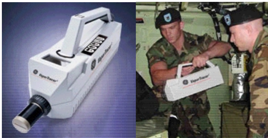
FIGURE 5.8 Military personnel using the IonTrack (now GE Interlogix) “sniffer,” which is capable of detecting drugs and explosives. It is based on ion trap mobility spectrometer (ITMS) technology. See http://www.geindustrial.com/ge-interlogix/iontrack/app_military.html .
