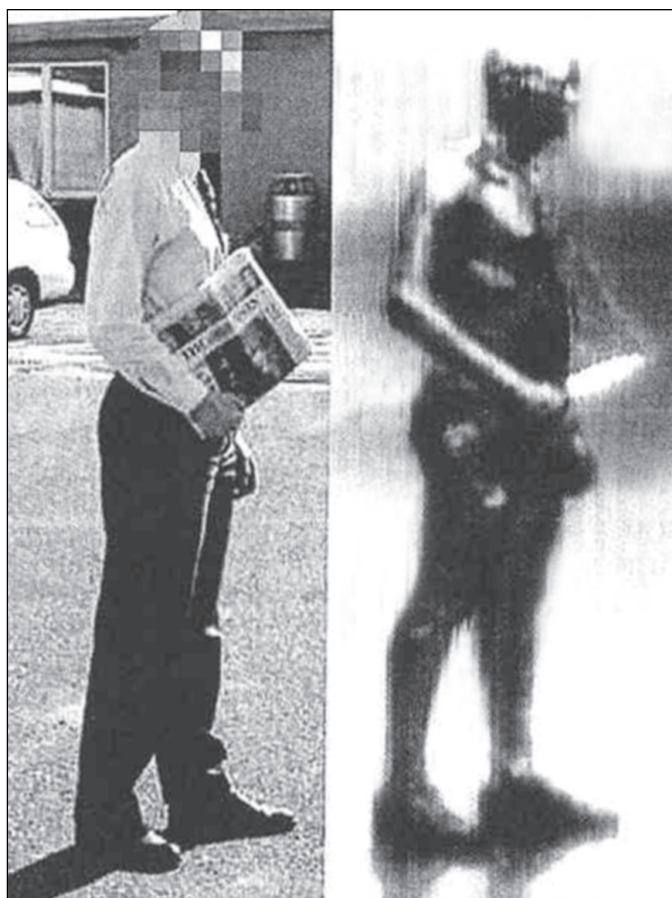
FIGURE 5.7 Visible and terahertz images of a man carrying a knife hidden in a newspaper and a gun in his pants. (QinetiQ.)
