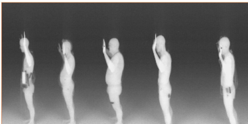
FIGURE 5.3 Standoff X-ray detection showing hidden explosives and other items on personnel. Images were taken from a van moving at 0.3 to 6 miles per hour using X-ray backscattering in “drive-by” mode. The mock suicide vest contained simulated C4 explosives and pipe bombs. Both the explosives and the pipe bombs are easy to see and are distinguishable from normal objects under clothing. (AS&E)
