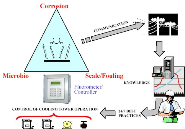
FIGURE 9.11 Automating the cooling water “triangle.”
