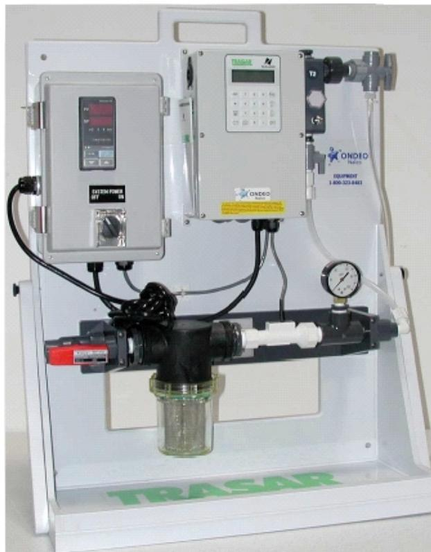
FIGURE 9.12 TRASAR for RO scale control.
