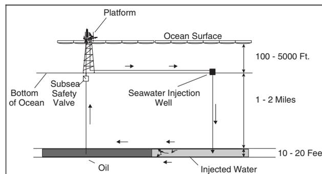
FIGURE 10.8 Nanofiltration membranes remove sulfate ions that could precipitate from water injected into oil reservoirs from offshore platforms.
