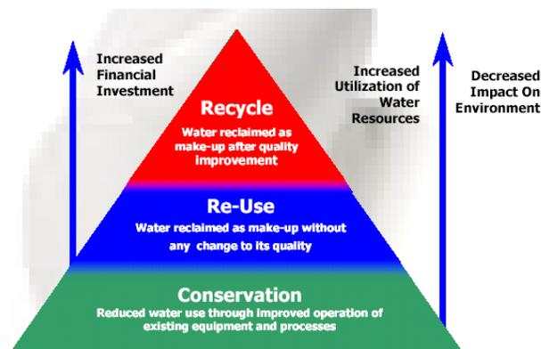
FIGURE 9.6 Water resource management and the Advanced Re-cycle Technology (ART™) services pyramid.
