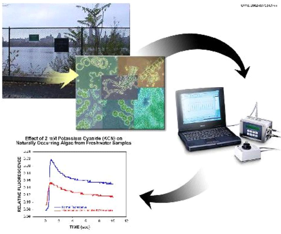
FIGURE 6.1 AquaSentinel: a continuous water monitoring system using naturally occurring algae as biosensors.
