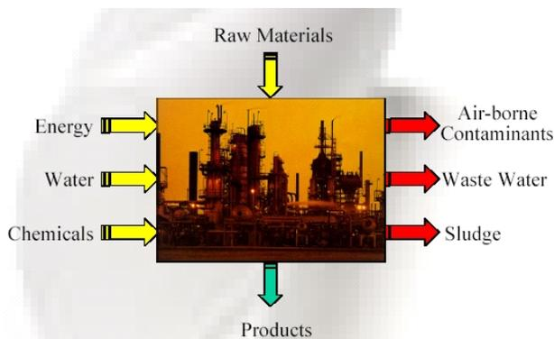
FIGURE 9.3 Industrial inputs and outputs.
