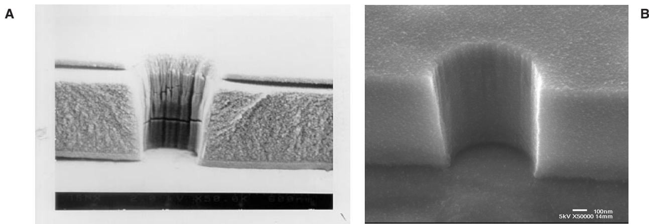
FIGURE 2.1 Comparison of a semiconductor component showing sidewall polymer (A) prior to cleaning, and (B) after cleaning with supercritical CO<sub>2</sub>.
