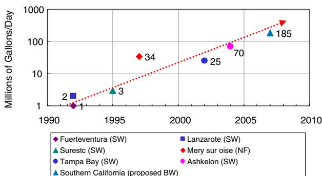
FIGURE 10.7 Reverse osmosis membrane facilities—largest plants as a function of time, with nanofiltration (NF), seawater (SW), and brackish water (BW).
