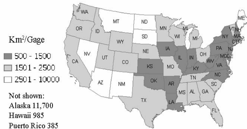
FIGURE 3-12 Density of NSIP gage locations measured in square kilometers of land area per gage. SOURCE: Based on USGS data ( http://water.usgs.gov/nsip ).
