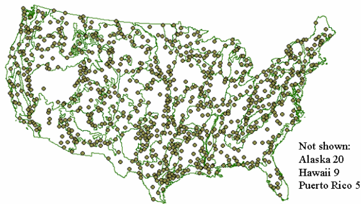
FIGURE 3-7 Gage locations for sentinel watersheds (874 gage sites of which 71 percent are solely for sentinel watersheds and 29 percent also serve other purposes). Lines shown are boundaries of ecoregions. SOURCE: Based on USGS data ( http://water.usgs.gov/nsip ).
