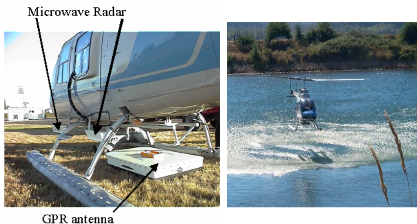
FIGURE 5-6 Helicopter experiments to measure discharge. SOURCE: John Costa, USGS, written communication, March 2002.
