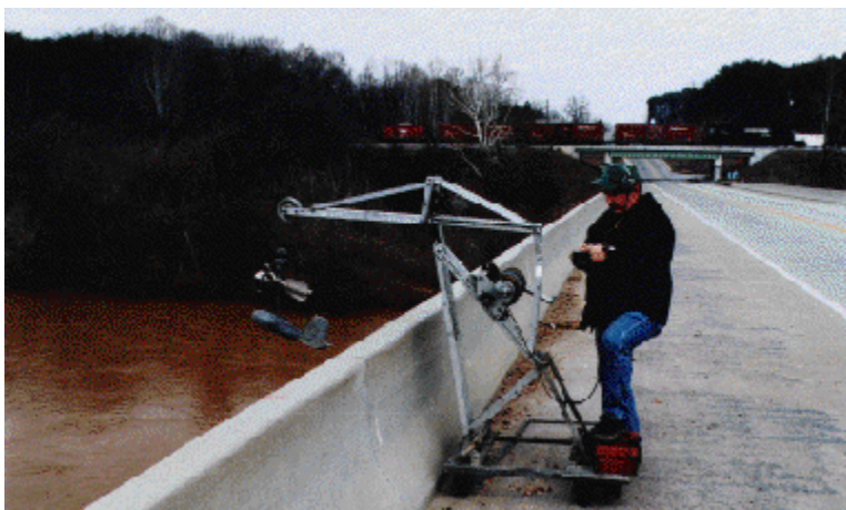
FIGURE 2-4 Measuring discharge by means of a bridge crane. The current meter, or “fish”, is lowered into the river to measure current velocity. The crane is wheeled along the bridge to obtain measurements at multiple sections. SOURCE: USGS ( http://water.usgs.gov/wid/FS_209-95/mason.figure.id.1.gif ).
