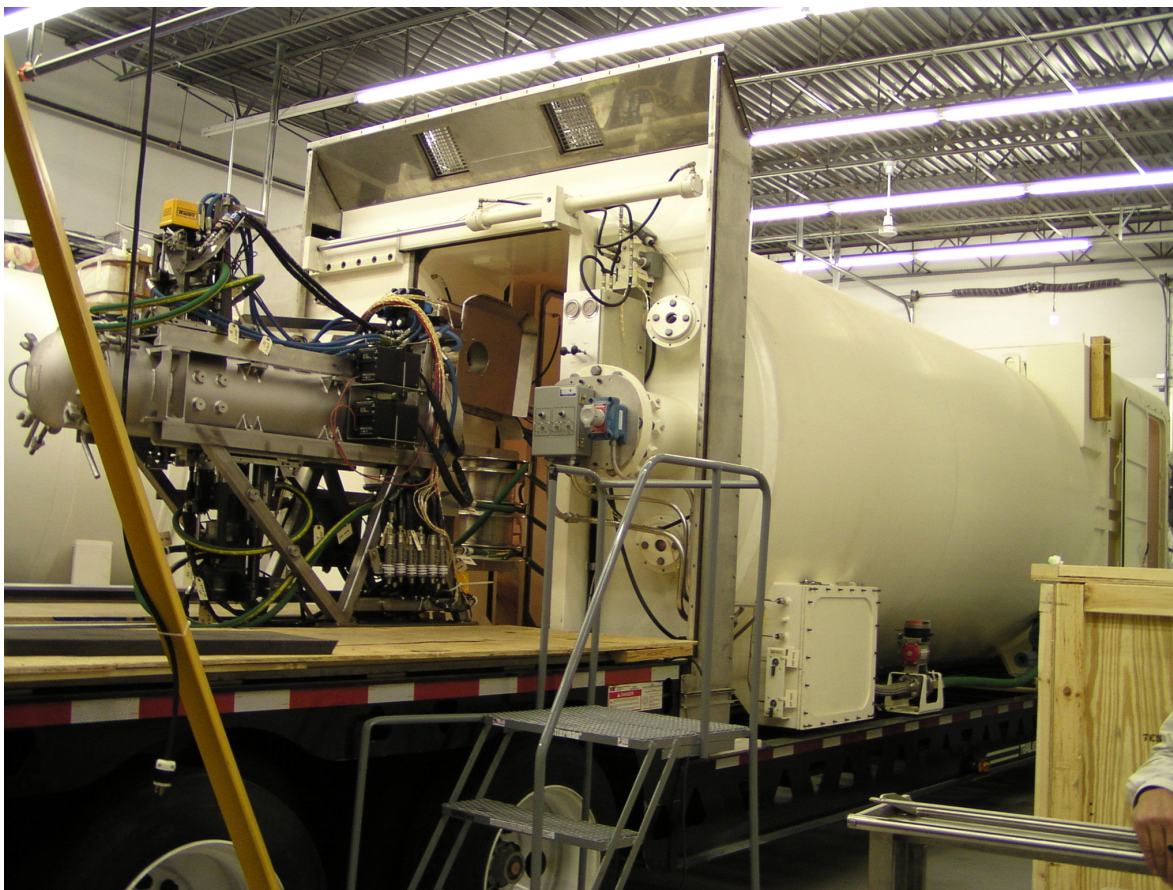
FIGURE 2-2 Auxiliary processing vessel removed from explosive containment chamber. Note the number of hoses, connections, etc. associated with the requirement to drill and drain munitions remotely when the APV (containing the munition) is inside the ECC containment vessel.
