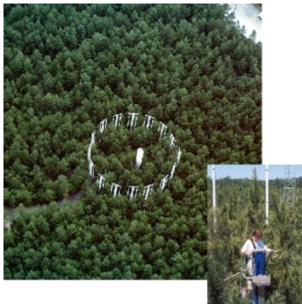
FIGURE 2-13 Free air CO 2 Experiment (FACE) is used to elucidate forest ecosystem responses to elevated CO 2 . A similar type of experimental approach could be used to better understand the long-term ecological effects of elevated pollutant concentrations. SOURCE: DOE 2001.
