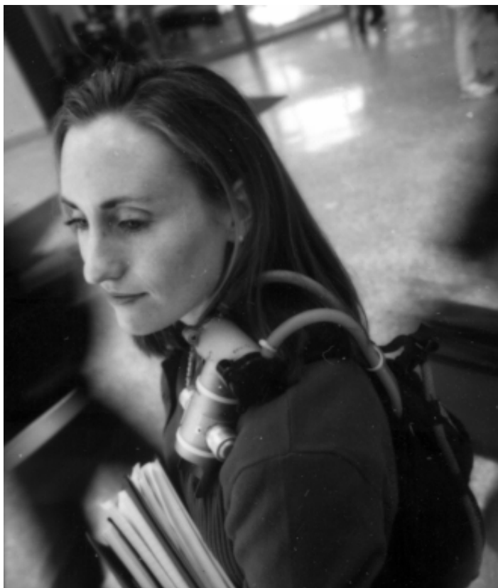
FIGURE 2-10 Volunteer wearing a personal exposure monitor to measure actual exposures to PM and gases during daily activities. SOURCE: HEI 2000. Reprinted with permission; copyright 2000, Health Effects Institute.
