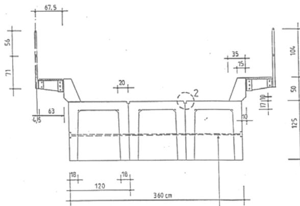
FIGURE 9 Channel-type girder railway bridge.
