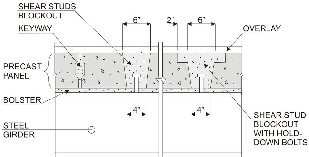
FIGURE 26 Longitudinal section, shear stud blockouts, and shear key. [Source: Babaei et al. (1).]
