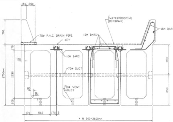
FIGURE 8 Box girder railway bridge.
