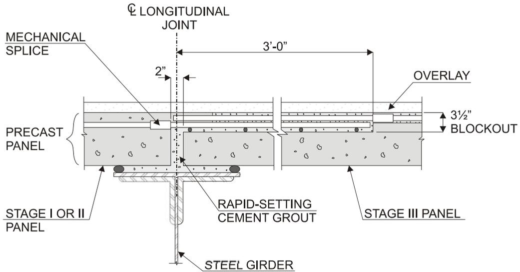
FIGURE 24 Longitudinal connections. [Source: Babaei et al. (1).]
