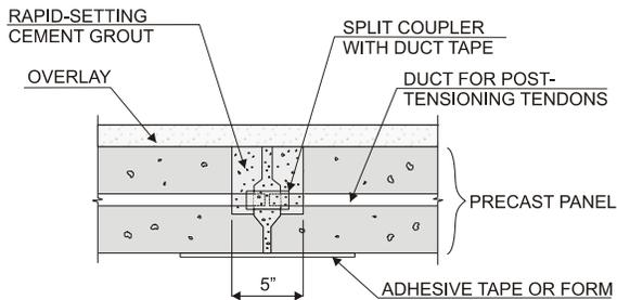
FIGURE 22 Posttensioning duct. [Source: Babaei et al. (1).]
