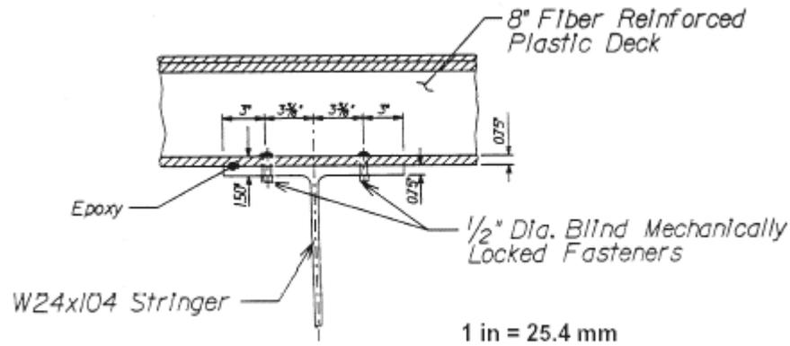
FIGURE 49 Deck to stringer connection using BOM blind bolts. [Source: Shekar et al. (34).]
