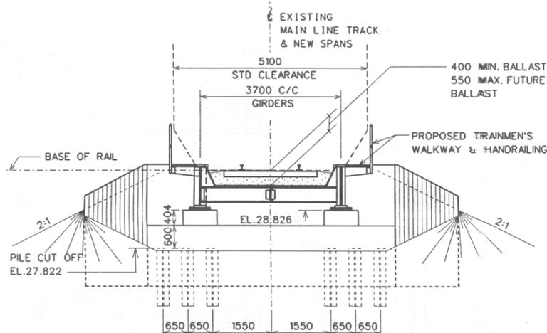
FIGURE 7 Through plate girder railway bridge deck.
