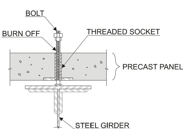
FIGURE 21 Leveling bolt system. [Source: Babaei et al. (1).]
