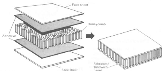
FIGURE 45 Sandwich construction.
