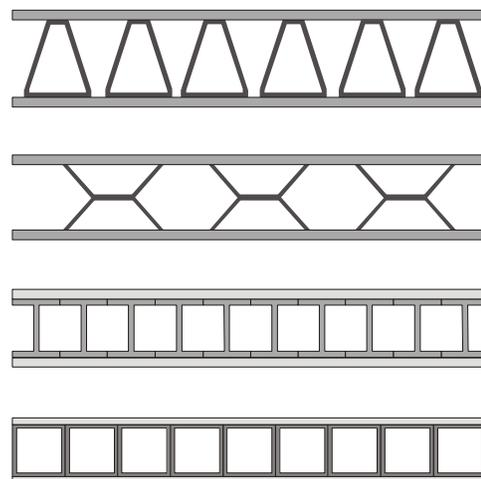
FIGURE 46 FRP decks produced from adhesive-bonded pultruded shapes.
