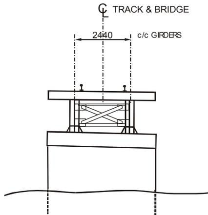
FIGURE 5 Open deck steel span railway bridge.
