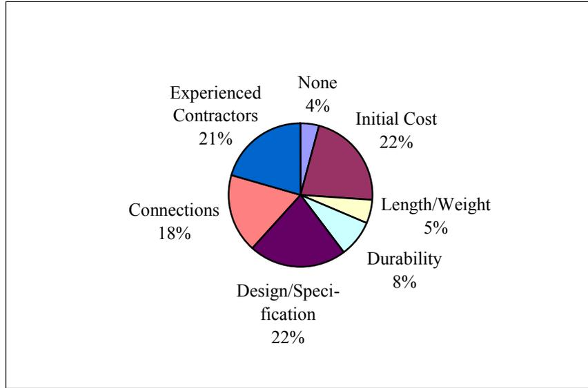
FIGURE 61 Aspects in bridge prefabrication requiring further development.
