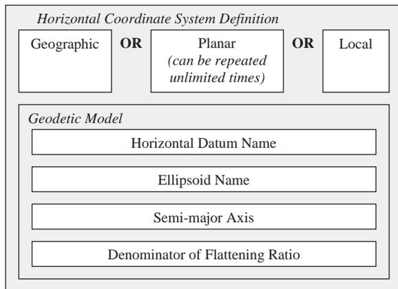
Figure 3-6. Current CSDGM horizontal coordinate system definition elements.
