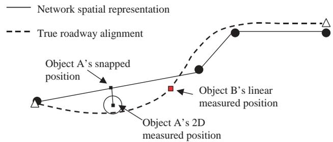
Figure 3-8. Transformation of 2D-measured position to LR position.
