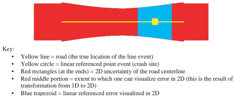
Figure 2-17. Combination of linear feature and 2D network.
