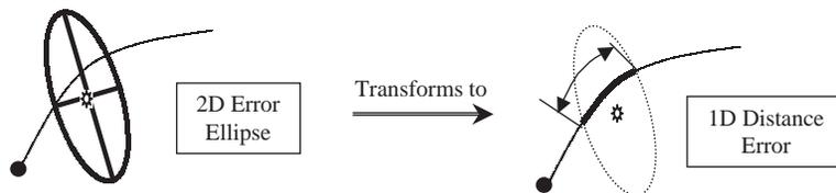
Figure 2-7. Example of 1D error generation.
