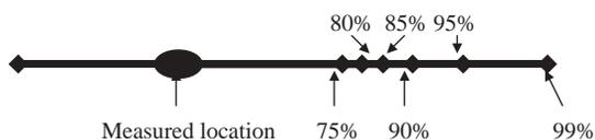
Figure 2-14. Probability zones of a one-dimensional point feature.
