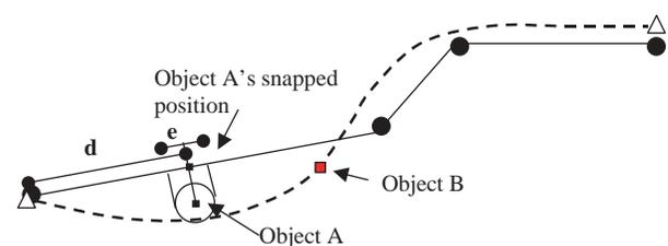
Figure 3-9. Transformation of nominal accuracy to distance error.
