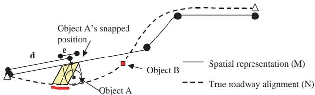
Figure 3-10. Projection of derived linear distance.
