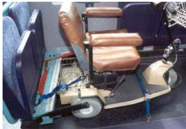
FIGURE 11 Forward-facing position in combi design, with two rear tie-downs and one strap over the footrest of the scooter.
