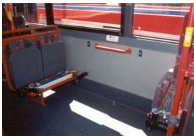
FIGURE 19 Combi system roadside in double-decker BC Transit low-floor bus.
