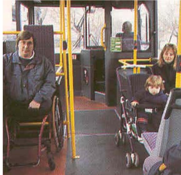
FIGURE 1 Transport for London rear-facing position with back panel and aisle stanchion.
