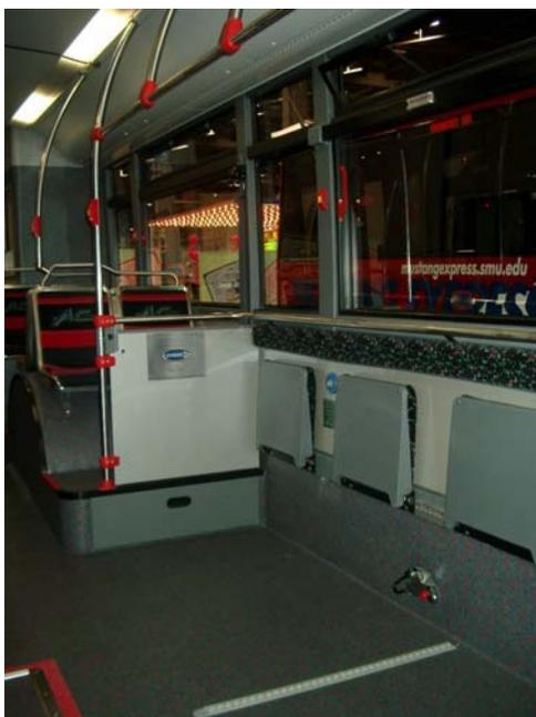
FIGURE 20 Forward-facing position (combi design) on prototype AC Transit BRT service bus.
