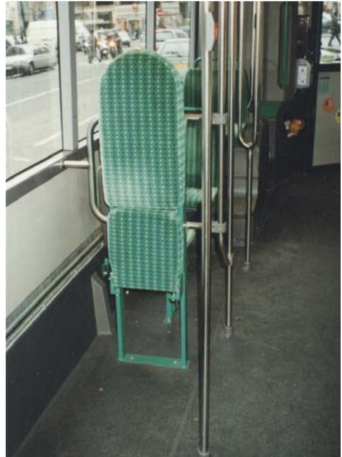
FIGURE 5 Paris (RATP) rear-facing position with flip-down seat built into back panel.
