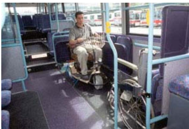
FIGURE 17 Combi 2 design for two travelers in the same position on BC Transit bus.
