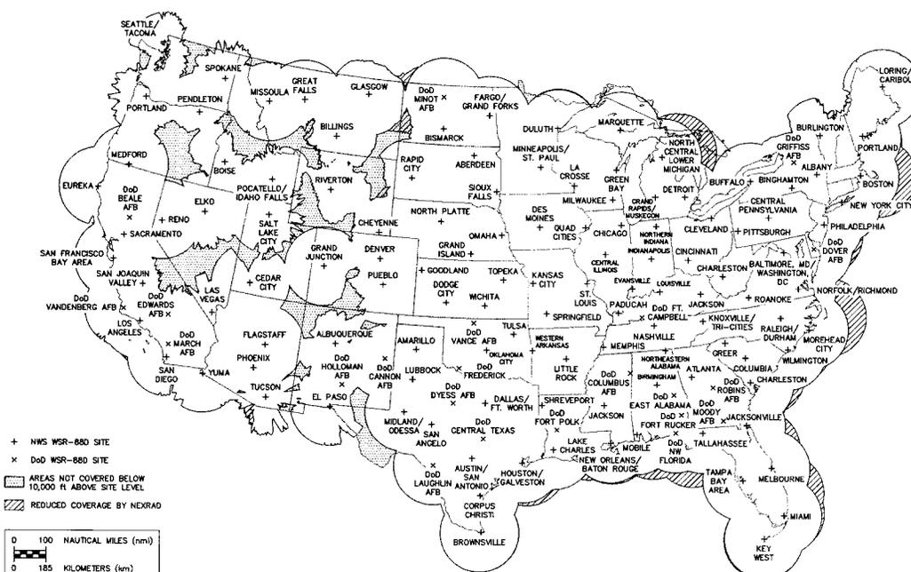
FIGURE C.1 Composite WSR-88D coverage at 3 km above site level for the contiguous United States and the locations of the NWS and DOD radar sites. Courtesy of SRI International (2003).
