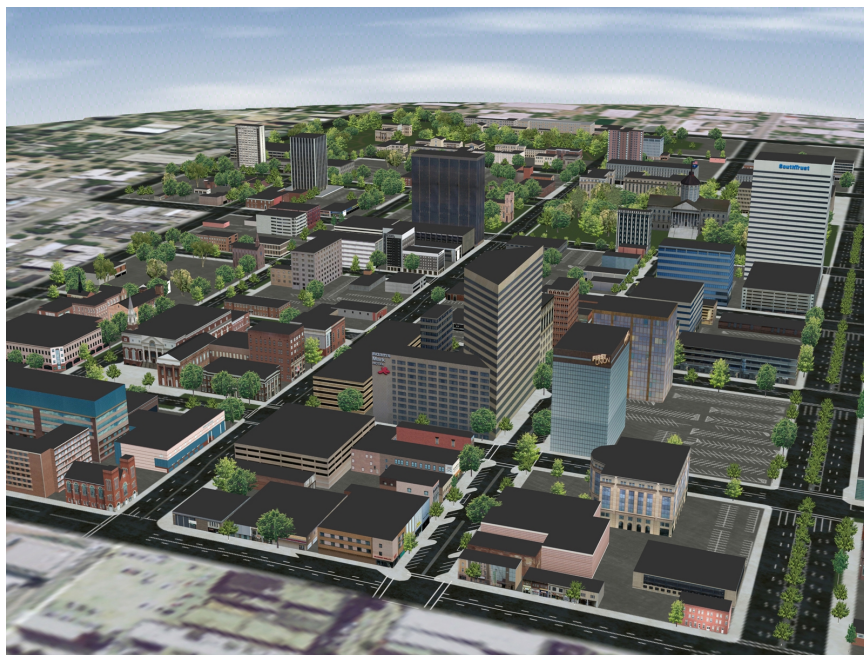
FIGURE 2.2 Urban three-dimensional model developed by Richland County, S.C., using advanced remote sensing/GIS techniques. Surface elevations, vegetation dimensions, and building outlines and heights were calculated using raw lidar points and high-resolution orthophotography. Building facade textures were added using oblique digital photography.
