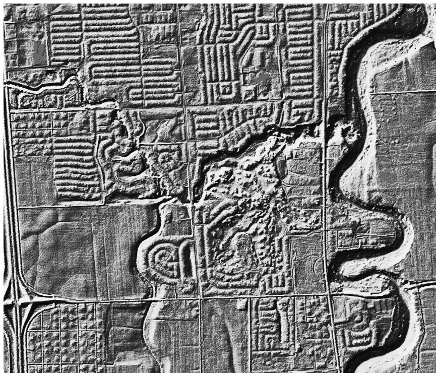
FIGURE 2.6 Lidar digital elevation model shaded relief map of the Red River Valley. SOURCE: North Dakota State Water Commission.
