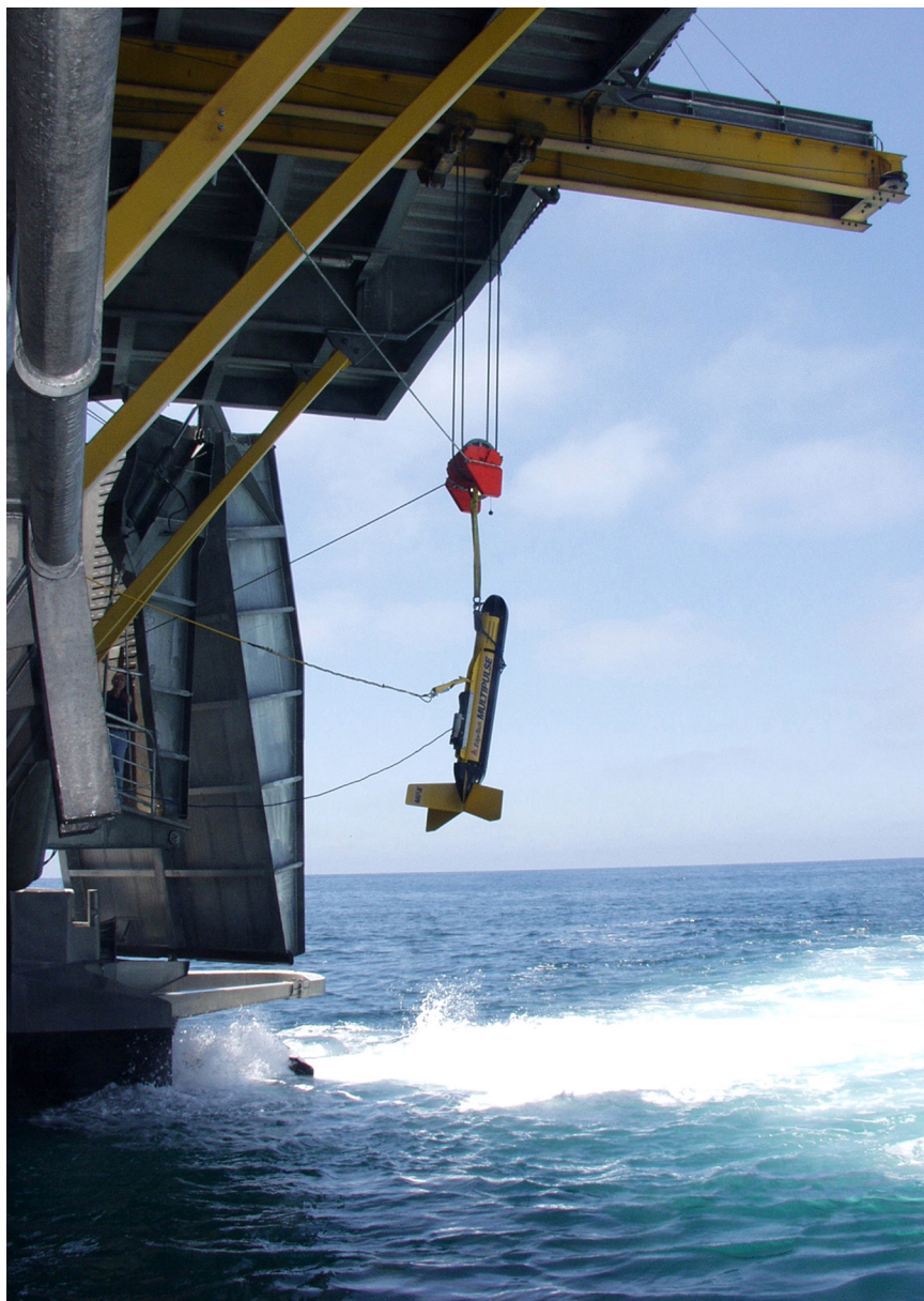
A side-scan sonar unit is lowered from the high-speed vessel Joint Venture (HSV-X1) into the waters off the coast of California during Fleet Battle Experiment Juliet. Sonar was used to locate underwater mines, to enable safe navigation of amphibious forces to reach the shoreline, during exercises in support of “Millennium Challenge 2002” (Photo courtesy of the U.S. Navy).
