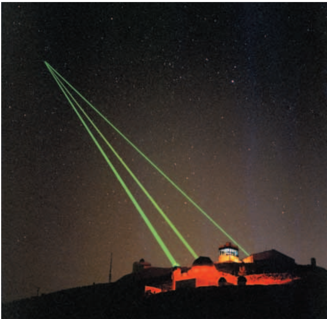
The night sky illuminated in a Guide Star demonstration. Inelastic scattering of the outgoing laser beams by the atmosphere makes them strikingly visible.
