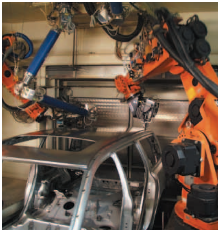
A CO 2 -laser-based automobile body welding station (2001).
