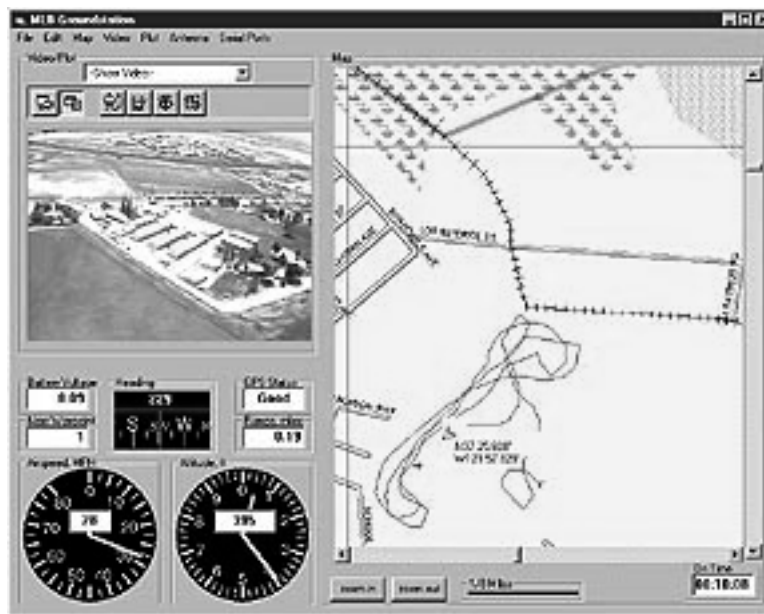
FIGURE 7 Ground station screen image. Source: Stephen Morris, MLB Company, Palo Alto, California.
