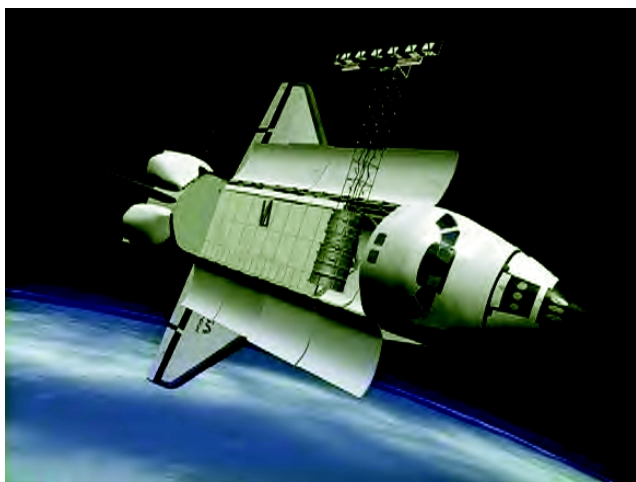
FIGURE 5-6 Artist's rendition of the SRTM 60-m (200-ft) mast being deployed from the space shuttle Endeavor (courtesy NASA Jet Propulsion Laboratory). Radar images are collected from the end of the mast and from the shuttle payload bay.
