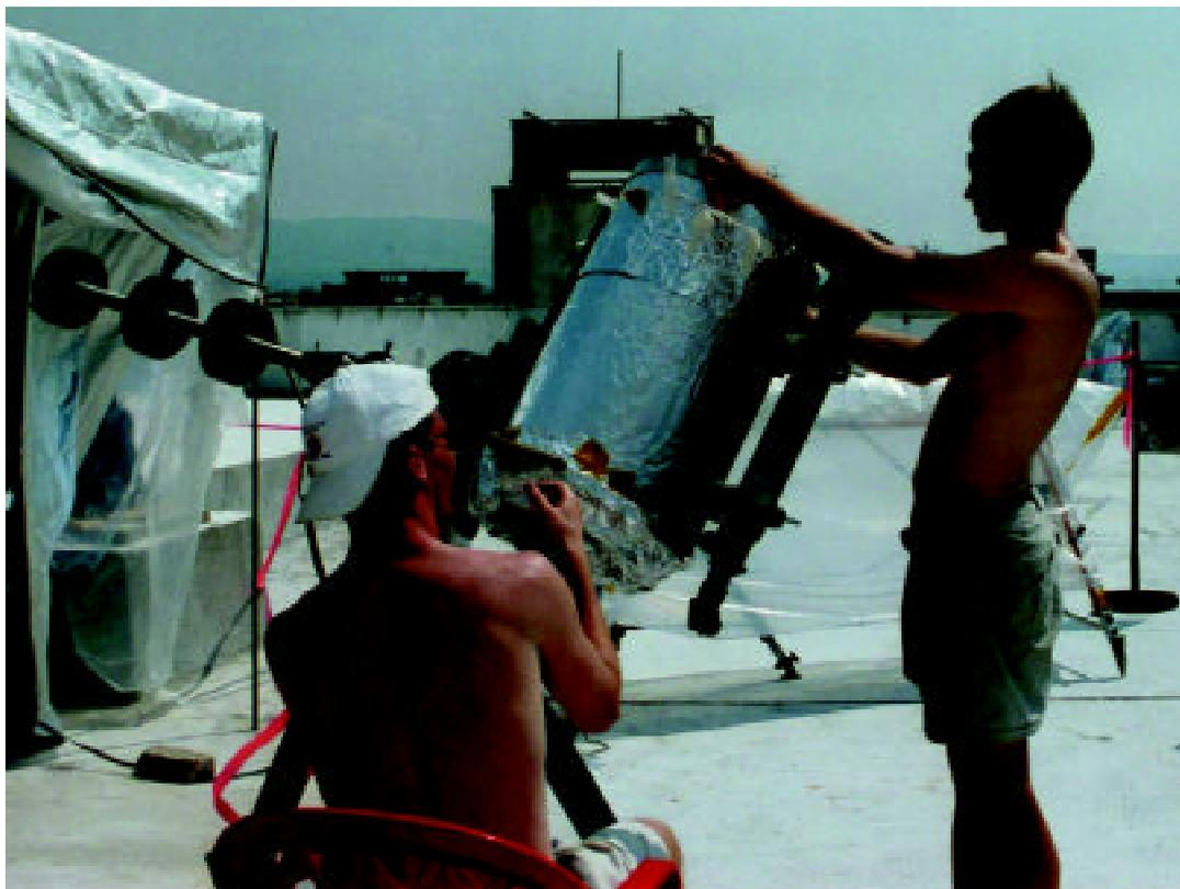
FIGURE 5.3 Two undergraduate students on the Williams College expedition to Rimnicu Vilcea, Romania, for the August 11, 1999, total solar eclipse. They are adjusting a 14-inch telescope for an experiment to detect coronal oscillations during the phase of totality. The expedition was supported in part by grants from the National Science Foundation, NASA, and the National Geographic Society's Committee for Research and Exploration. Photograph courtesy of J. Pasachoff (Williams College).
