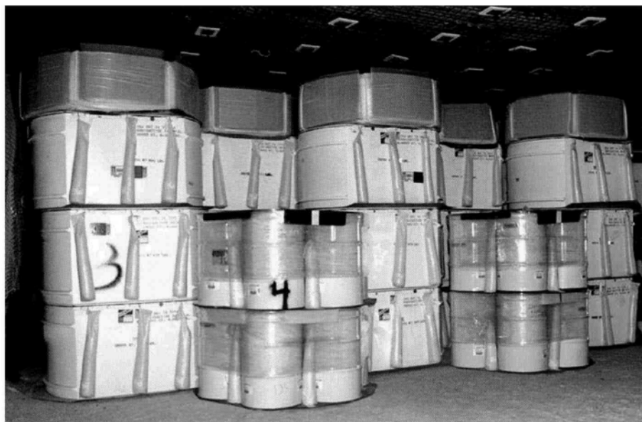
Figure 3.1 Standard waste boxes and packs stacked in one room of the WIPP repository. Notice the layers of plastic film around the drums. SOURCE: DOE, 2000d.
