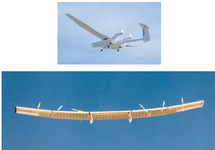
FIGURE 3-3 Unconventional designs with challenging configuration aerodynamics. Top: Aurora Flight Science Corporation's Theseus. Bottom: AeroVironment Pathfinder. Source: NASA.
