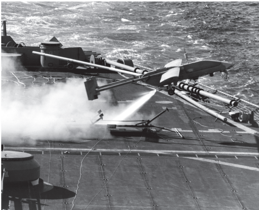
FIGURE 1-1 Pioneer UAV taking off from the deck of the USS Iowa . Source: Pioneer UAV, Inc.
