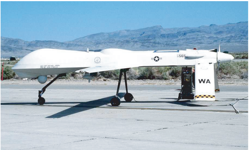
FIGURE 1-3 Predator airborne surveillance, reconnaissance, and target acquisition vehicle. Source: Air Combat Command, U.S. Air Force.
