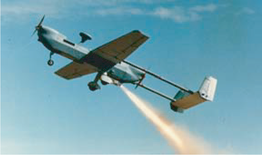
FIGURE 1-2 Hunter reconnaissance and surveillance UAV. Source: Director, Operational Test and Evaluation, U.S. Department of Defense.
