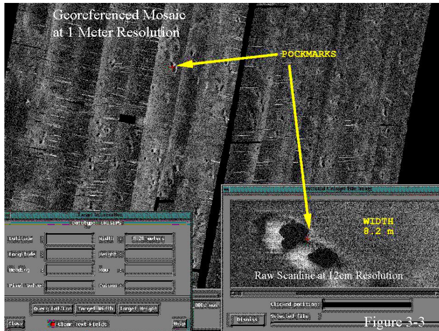
FIGURE 3-3 An acoustic imagery mosaic with one meter resolution. On this image numerous “pockmarks” can be seen. These features are likely to have resulted from seafloor release of hydrocarbon gases.
