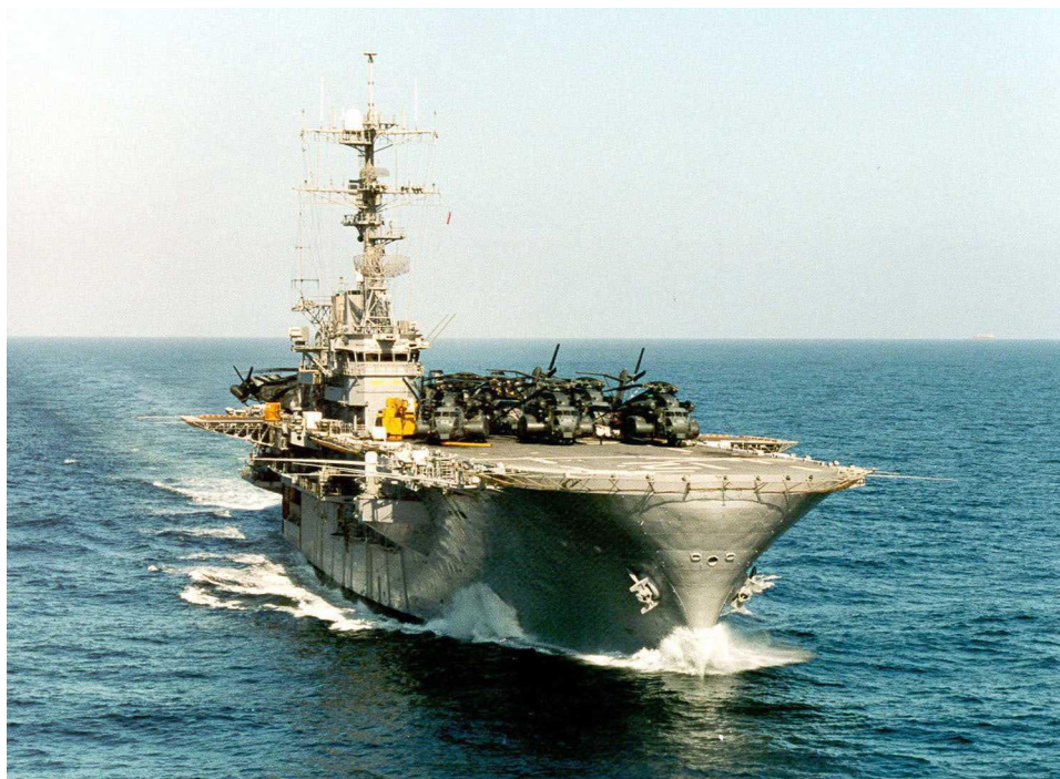
FIGURE 2-4 The USS Inchon provides support for sustained mine countermeasure (MCM) operations by furnishing a landing platform for MH-53E Sea Dragon minesweeping helicopters while also acting as a repair and re-supply facility for Avenger and Osprey class coastal minehunters.
