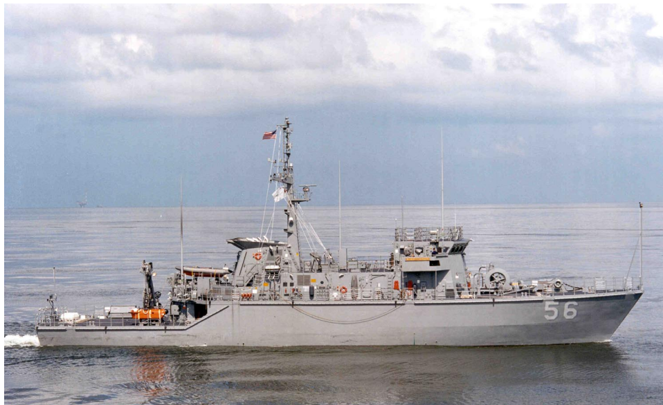
FIGURE 2-6 The Osprey class has a shorter endurance than the Avenger and is more operationally capable due to its lower acoustic and magnetic signature. The Osprey only has a minehunting capability. Osprey class ships are constructed from glass-reinforced plastic (GRP) fiberglass.
