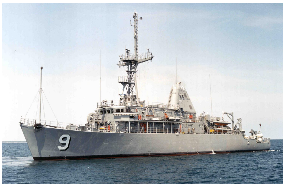
FIGURE 2-5 The Avenger class of minesweeper was designed to find, classify, and destroy moored and bottom mines in both coastal and offshore areas. This class has added capabilities to conduct mechanical, acoustic, and magnetic mine sweeping. The ships have a fiberglass-sheathed wooden construction to make the hull less detectable by influence mines.
