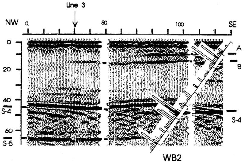
FIGURE 3.2 Semihorizontal fracture zones observed by ground penetrating radar along a profile measured on granitic outcrops at the Underground Research Laboratory, Manitoba, Canada, showing distribution of fractures along borehole WB2. Reflectors S-4 and S-5, seen at depths of 40 to 50 m and 65 m, respectively, are verified by increased fracture frequency observed in the slanted borehole. (From Holloway et al., 1992).
