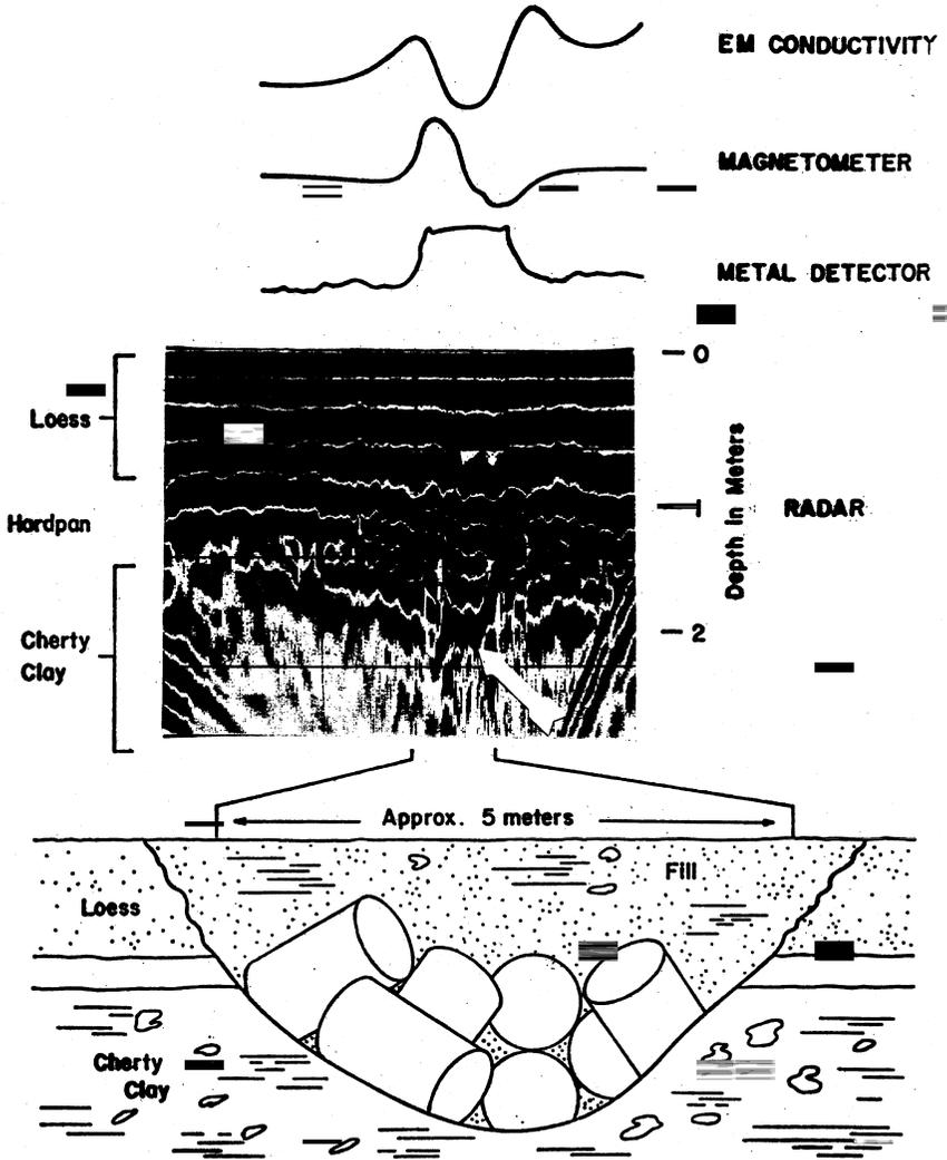
FIGURE 3.6 Buried metallic drums with representative magnetic and EM signatures; GPR signals show disturbed ground and surrounding stratigraphy. (After Benson and Glaccum, 1980.)
