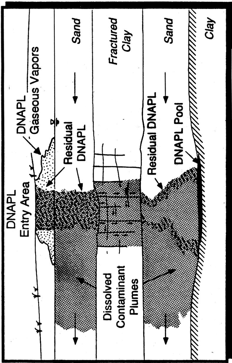
FIGURE 3.5 Schematic representation of PCE in an aquifer of sand and fractured clay. Some of the PCE volatilizes, some is trapped as a residual in soil pores, some migrates into the fractures, and some pools on the clay layers (from Cohen and Mercer, 1993).
