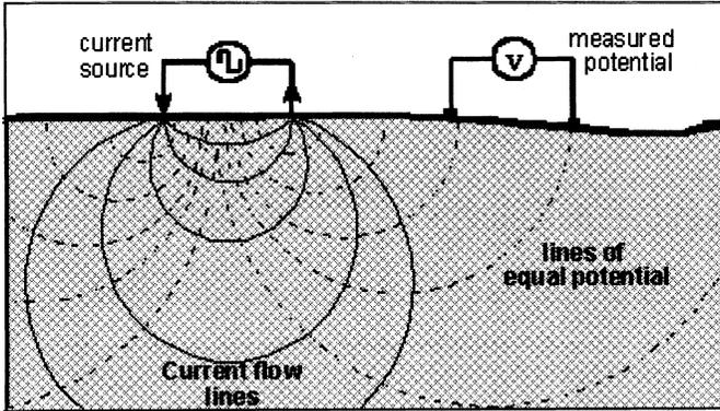
FIGURE 4.2 Schematic of a resistivity survey.
