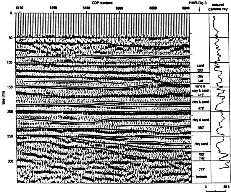
FIGURE 4.9 Seismic reflection profiling for geological variability.
