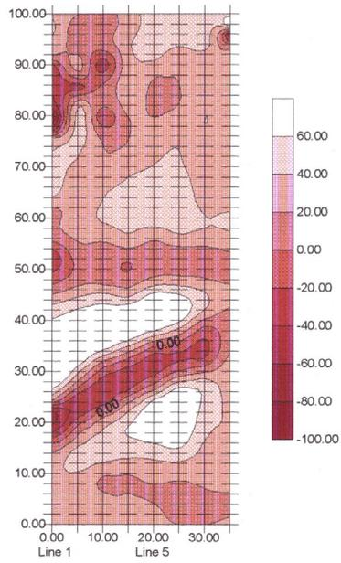
Map view of a different location showing a previously unknown pipeline (lower left to upper right) at an angle to the main pipeline as above (horizontally across the top). It was found to be another pipeline of a previous vintage and purpose that had not been removed. Line spacing is 5 feet; all other details are the same as the top figure. North is to the left.
