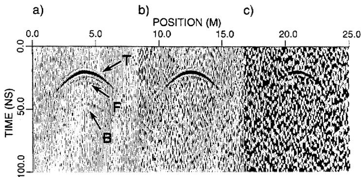
FIGURE 5.3 Visibility of GPR reflections decreases as the signal-to-noise (S/N) ratio increases; (a) is for S/N of 15.0, (b) for S/N of 7.5, and (c) for S/N of 1.5. T is the reflection from the top of a buried tank, B from the bottom of the tank, and F from a fluid (air/gasoline) interface inside the tank. Figure is from Zeng and McMechan (1997).
