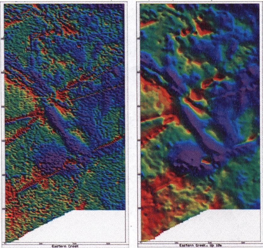
Magnetic data collected with a hand-held total-field magnetometer with resolution of 0.02 nT on traverses recorded with the sensor 1 m above ground with a sample interval of 0.5 m and a line spacing of 10 m, over an area 700 m by 1400 m. The data show a wealth of geological detail, containing shear zones, very thin dikes (<1 m), and a reverse magnetized plug.
