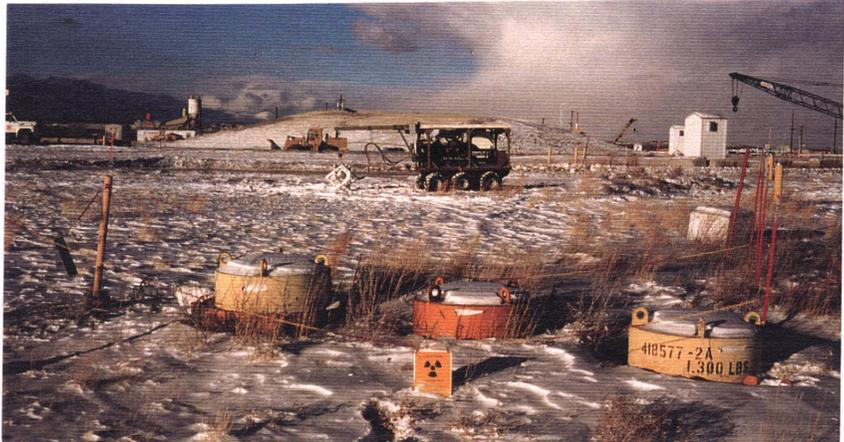
Photograph shows a survey being conducted at a site at a radioactive waste management acid pit at the Idaho National Engineering Laboratory. The site had been used for dumping acid that contained radioactive wastes and other contaminants. This was an operational survey to provide information for remediation of the site, and the precise location of the wastes were not well known.
