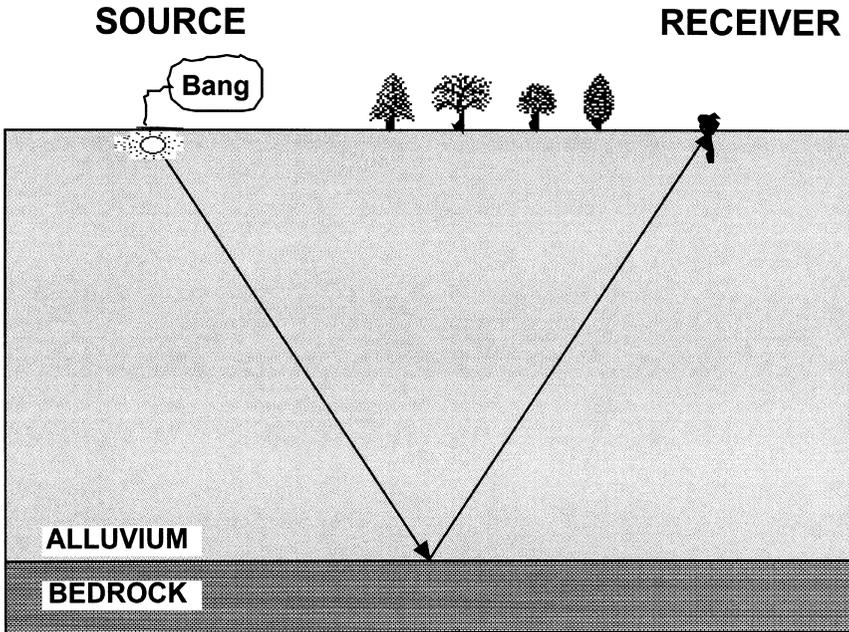
FIGURE 4.6 Simple reflection from bedrock. Either a seismic wave-velocity contrast or a mass density contrast is required for seismic waves to be reflected from the geological interface.
