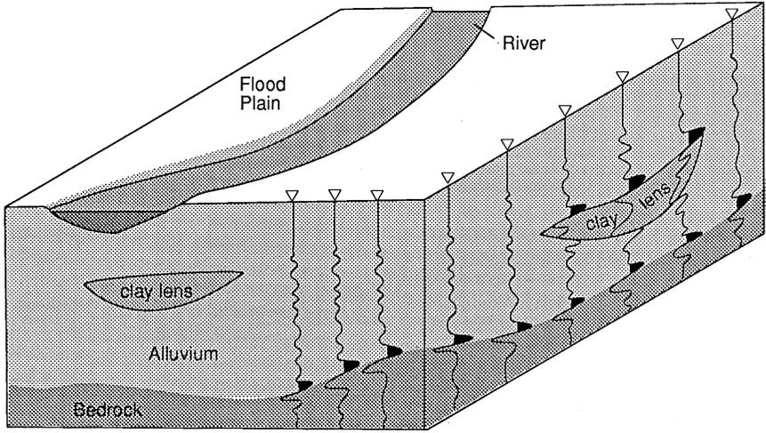
FIGURE 4.5 Simplified cartoon showing the “mapping” of bedrock and other features by seismic waves traced to individual geophone receivers.
