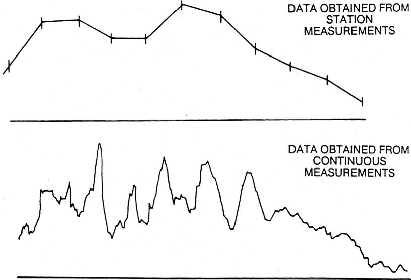
FIGURE 3.4 Comparison of station and continuous surface EM conductivity measurements made along the same transect. The electrical conductivity peaks are due to fractures in gypsum bedrock. (From Benson et al., 1982.)
