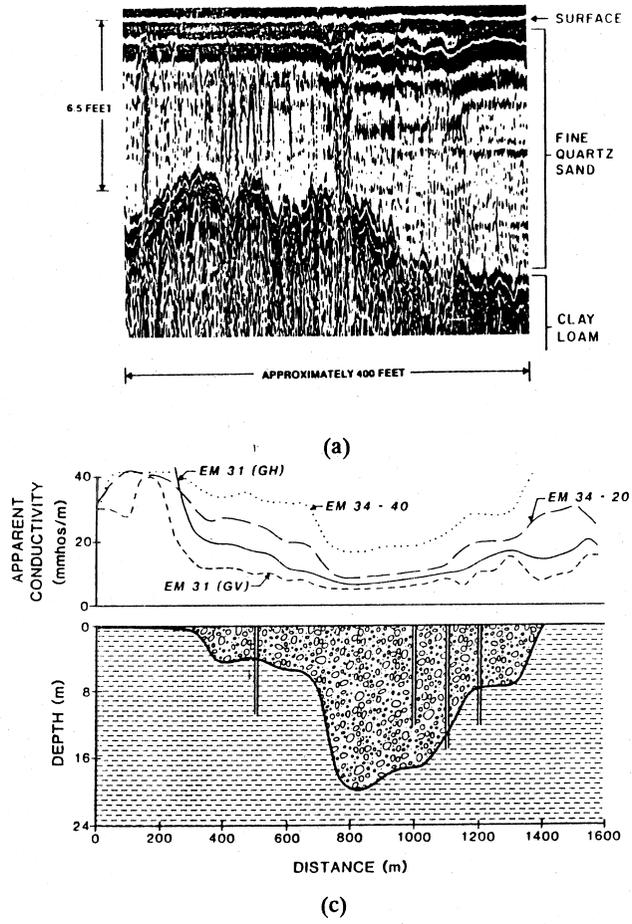
FIGURE 3.1 Examples of stratigraphic interpretations using subsurface geophysical surveys: (a) ground penetrating radar (from Benson et al., 1982); (b) delineating a bedrock channel by seismic reflection (from Benson, 1991); (c) relationship of EM
