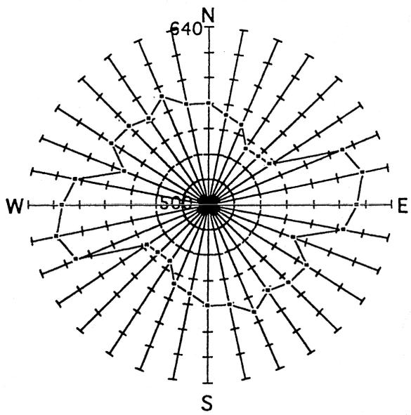
FIGURE 3.3 Resistivity measurements made in 16 different directions define a resistivity ellipse whose major axis is aligned with the fracture orientation. This example, from an open-pit quarry in southern Indiana, demonstrates that the dominant fracture direction is east-west. (From Cohn and Rudman, 1995.)
