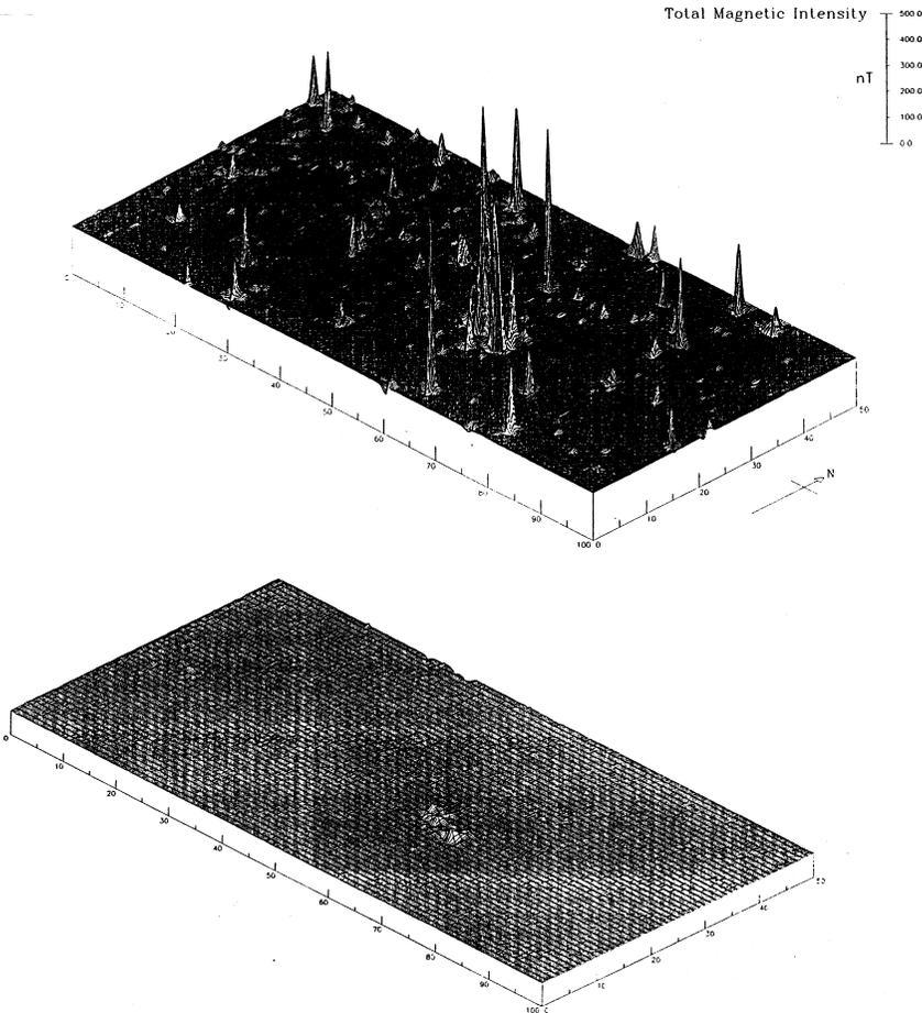
FIGURE 2.2 High-resolution magnetic survey for UXO detection
