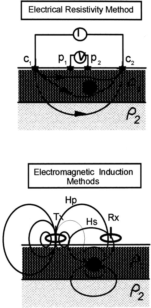
FIGURE 4.1 Simple comparison of electrical resistivity methods and electromagnetic induction (EM) methods. EM methods are generally noncontact, whereas resistivity methods require driving metal electrodes into the ground.
