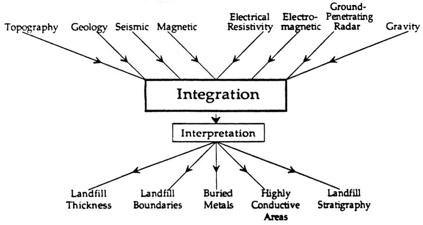
FIGURE 5.1 Schematic diagram of the concept of integrating geologic information and data from diverse geophysical methods for determining properties of a landfill. (After Roberts et al., 1989.)
