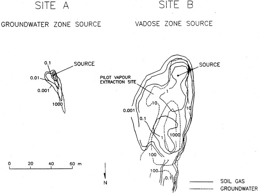
FIGURE 2.1 Areal extent of soil gas and groundwater contamination derived from TCE (trichloroethelene) emplaced below the water table (site A) and in the vadose zone (site B). (all units in grams per liter.) Figure from Rivett and Cherry (1991), which should be referred to for additional details.
