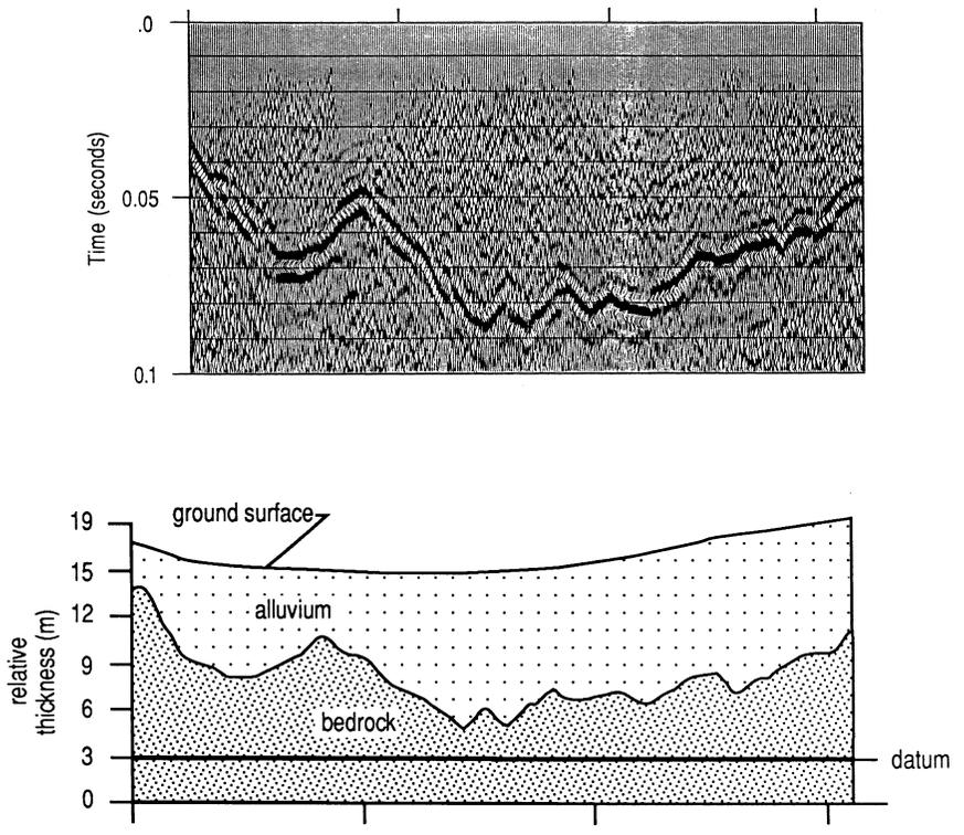
FIGURE 4.8 Seismic reflection cross section and interpreted cross section. The purpose of the characterization was to determine the placement of a monitoring well, which was designed to be placed at the deepest bedrock-alluvium contact. From D. Steeples.
