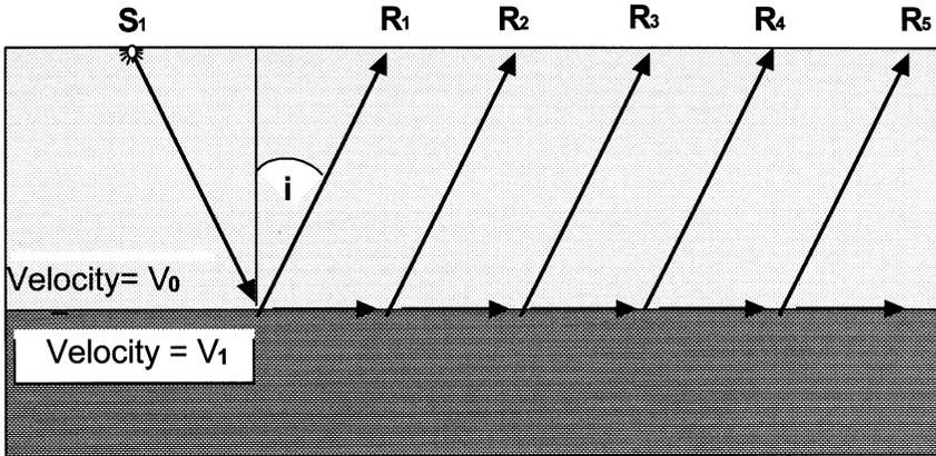
$$\sin i = V_0/V_1$$
