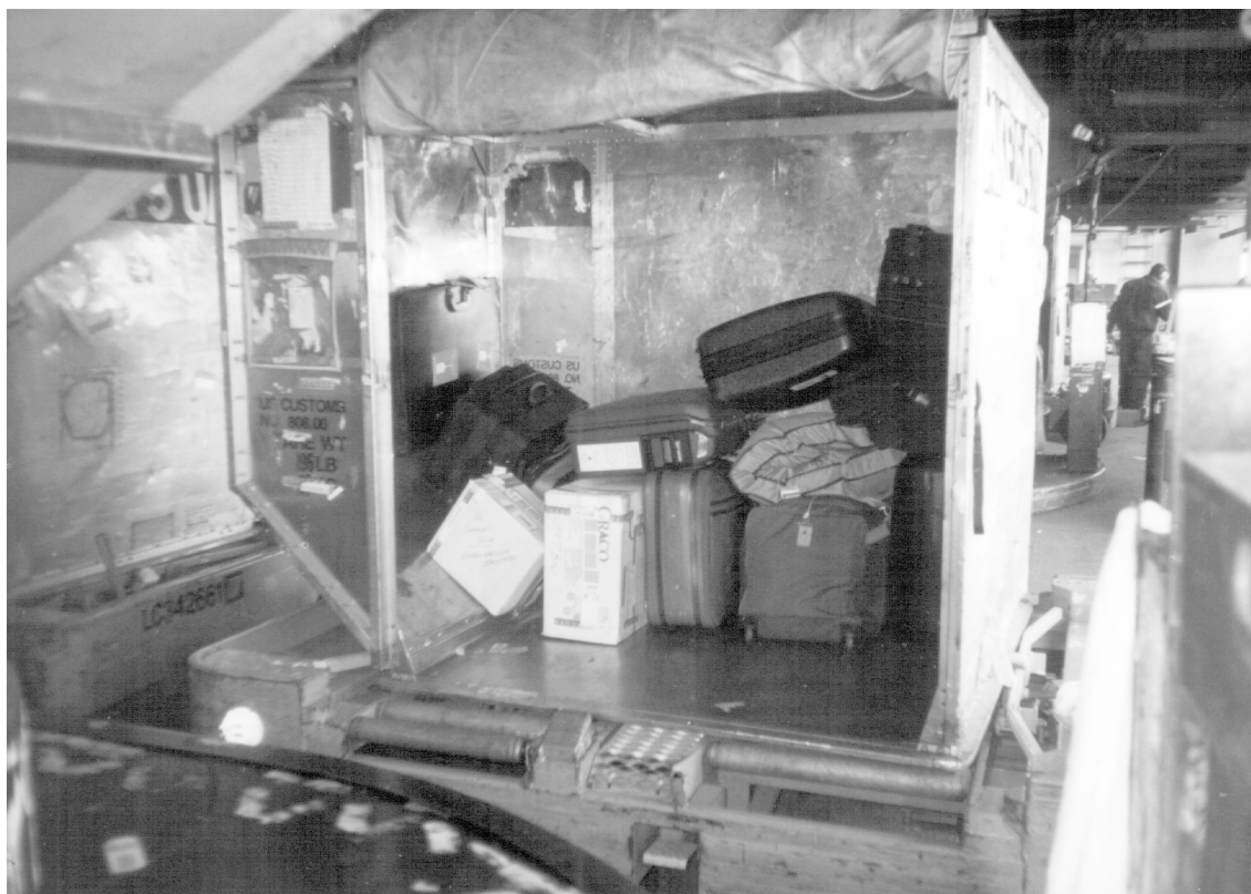
FIGURE 4-6 Typical LD-3 container.
