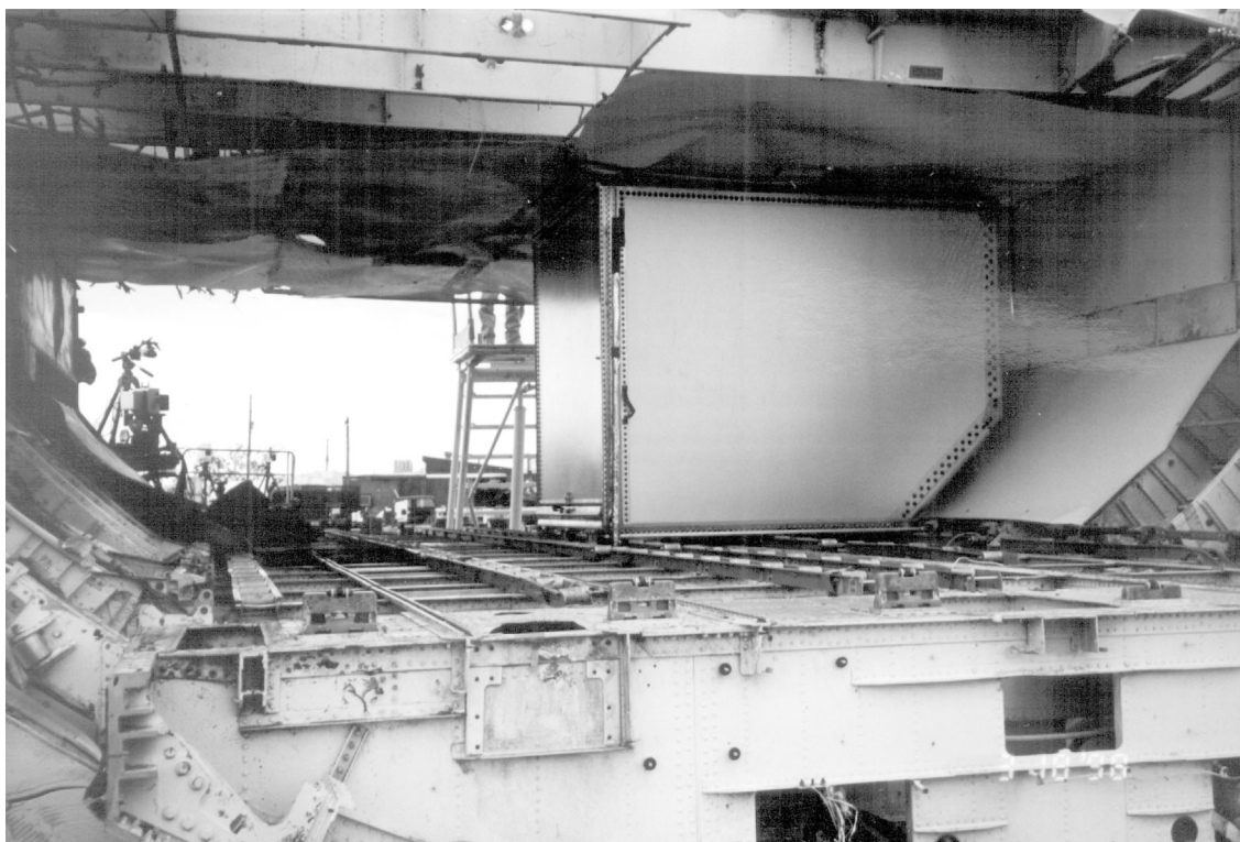
FIGURE 5-2 Galaxy HULD in test position prior to blast test.
