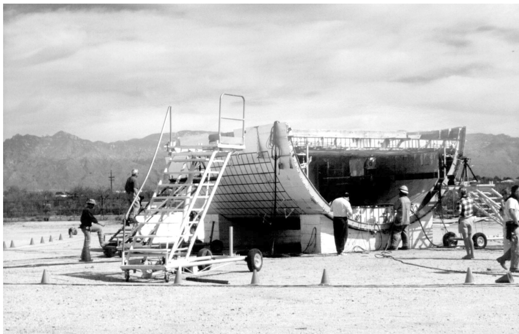
FIGURE 5-1 Cargo hold for blast testing HULDs.
