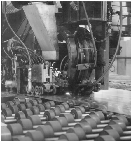
Automated welding system for the production of door inner blanks. Source: TWB Company.
