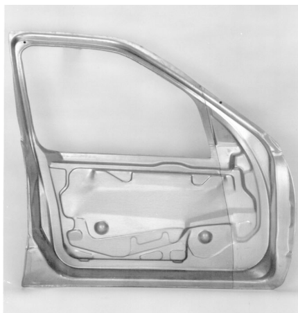
Laser-welded door inner panel. Source: TWB Company.
