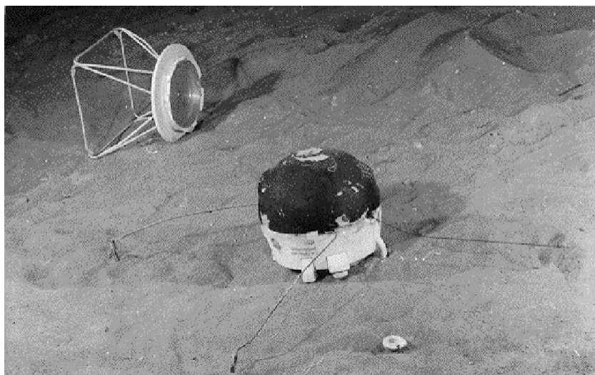
FIGURE 3.4.1 Hopping is an appealing means of providing mobility in a low-gravity environment. The former Soviet Union planned to use hoppers to undertake multipoint measurements on the martian moon, Phobos, in the late 1980s as part of the ambitious, but unsuccessful, Phobos program. Although their parent spacecraft failed before they could be released, these 60-cm-by-90-cm (approximate) hoppers were designed to leap from one site to another up to 20 m away and were outfitted with an array of scientific instruments, including an x-ray fluorescence spectrometer, a magnetometer, and a gravimeter. The two mechanical rods used to position the device are visible to the left of the semispherical hopper. This photograph of one of the engineering test models and its mounting adaptor (upper left) is courtesy of Valery Gromov and Alexander Zakharov.
