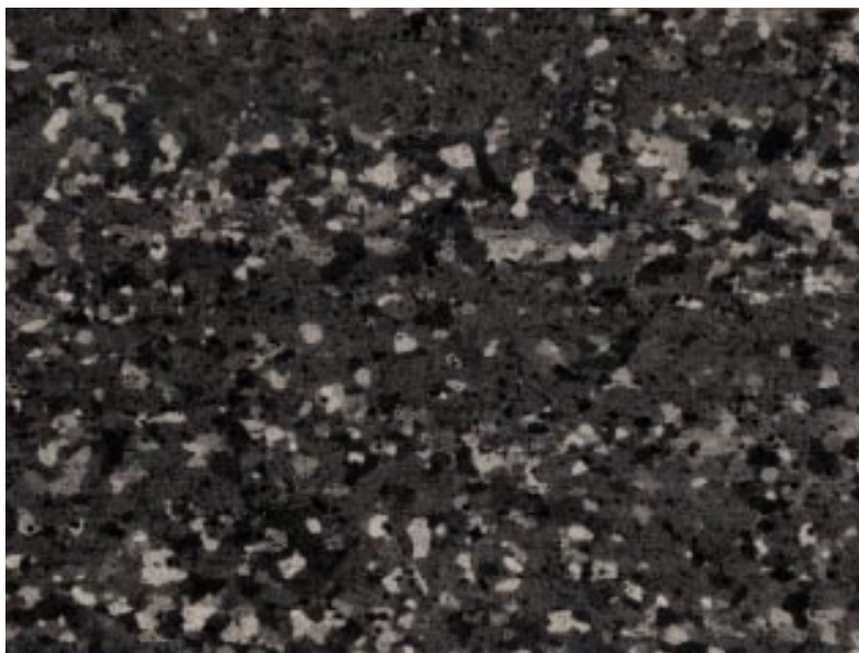
FIGURE 1 Metal microstructure composed of crystals. SOURCE: Reprinted with permission from The Minerals, Metals and Materials Society and ASM International (Beaudoin et al., 1998).
