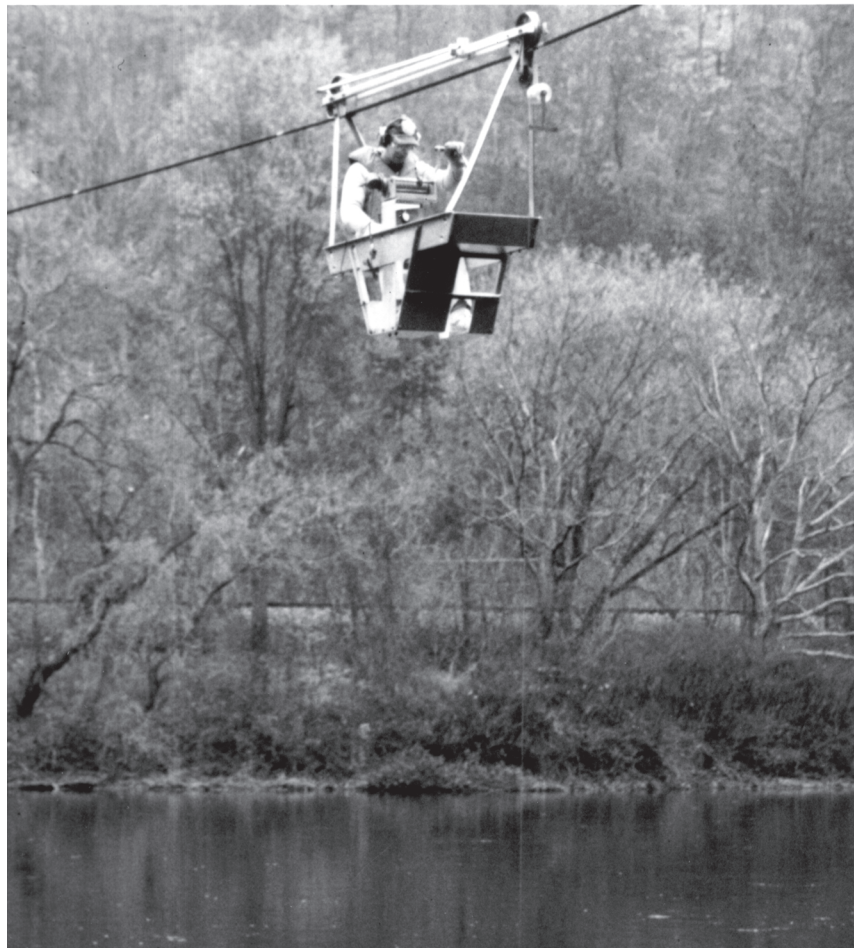
Discharge measurements are especially important during extreme flow events, even though conditions are least favorable. Photo courtesy of U.S. Geological Survey.
