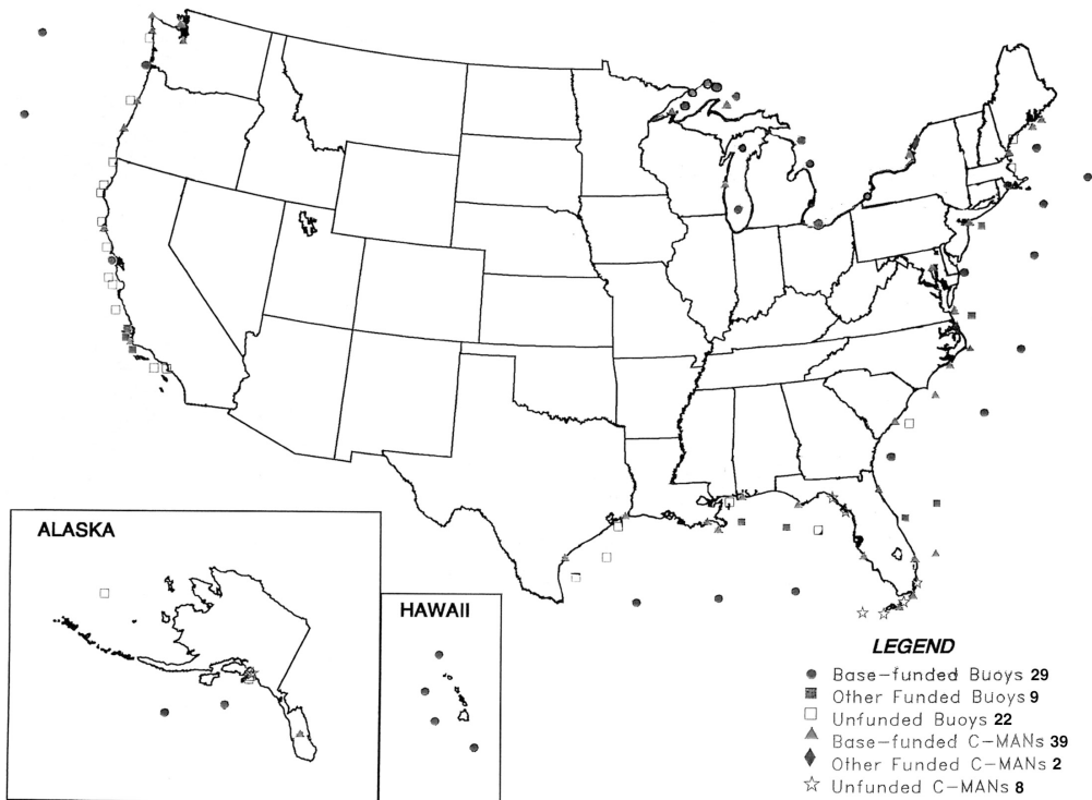
FIGURE 6 Distribution of existing NOAA base-funded moored buoys and C-MAN stations shown in Fig. 5 plus the additional NOAA unfunded stations that together make up the current moored buoy and C-MAN station network. (Source: U.S. Department of Commerce, National Oceanic and Atmospheric Administration-Marine Weather Services)
