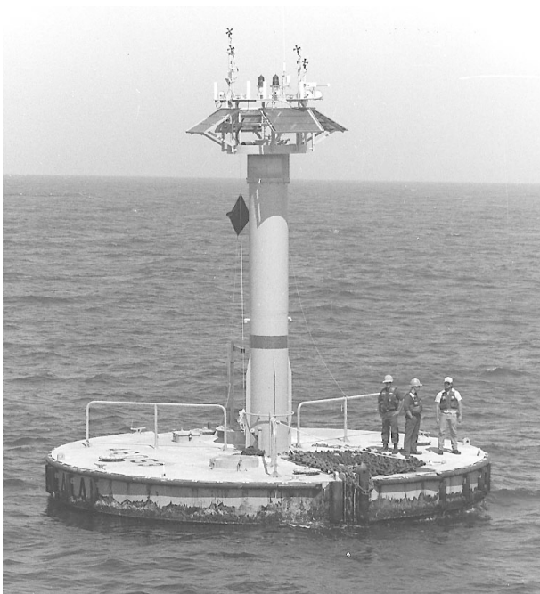
FIGURE 15 Pictures of representative moored buoy types deployed in the Alaska/Bering Sea (12-meter discus), mid-Gulf of Mexico (10-meter discus), Hawaii (6-meter NOMAD), and Great Lakes (3-meter discus) regions. (Source: U. S. Department of Commerce, National Oceanic and Atmospheric Administration)
