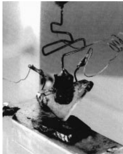
FIGURE 1.1 The world's first transistor, developed in 1947. It was a point-contact device roughly one centimeter across. (Courtesy of Lucent Technologies Bell Laboratories.)
