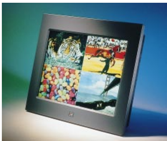
FIGURE 2.10 A high-resolution, active-matrix liquid crystal flat-panel display. (Courtesy of dpiX, Incorporated.)
