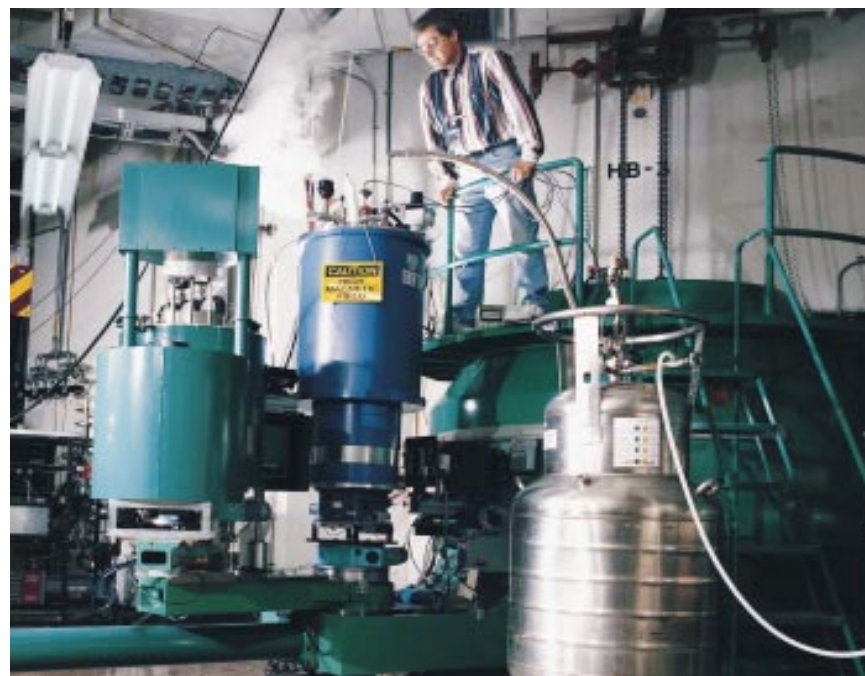
FIGURE 4.4 The High Flux Isotope Reactor provides the nation's most intense steady-state neutron beams for materials research and isotope production. The neutron scattering spectrometer shown here is being configured for an experiment that uses the neutron's unique sensitivity to magnetism. (Courtesy of Oak Ridge National Laboratory.)
