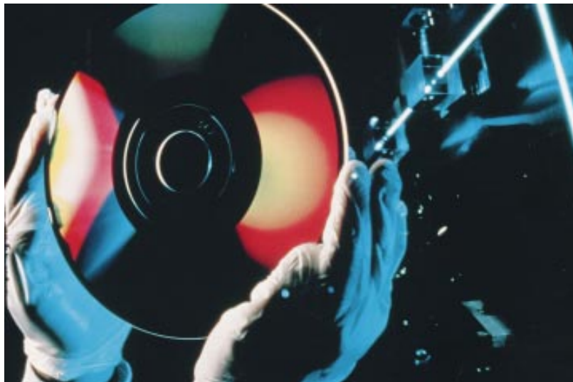
FIGURE 2.4 A magneto-optical disk. Information is stored magnetically and read out optically. (Courtesy of IBM Research.)
