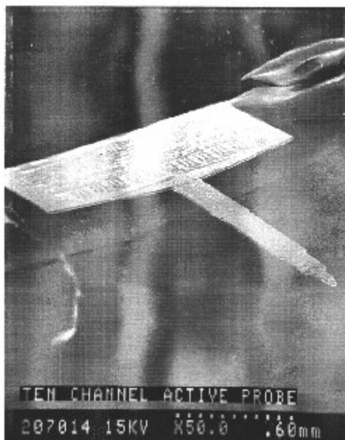
FIGURE 2-4 Multichannel neural probe with integrated electronics fabricated by the dissolved-wafer process. Source: Najafi and Wise, 1986.
