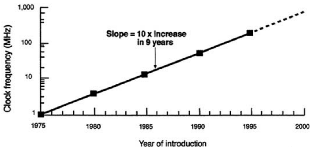
FIGURE 5-3 Operating frequency of high-end microprocessors used in desk-top computers by year of introduction.
