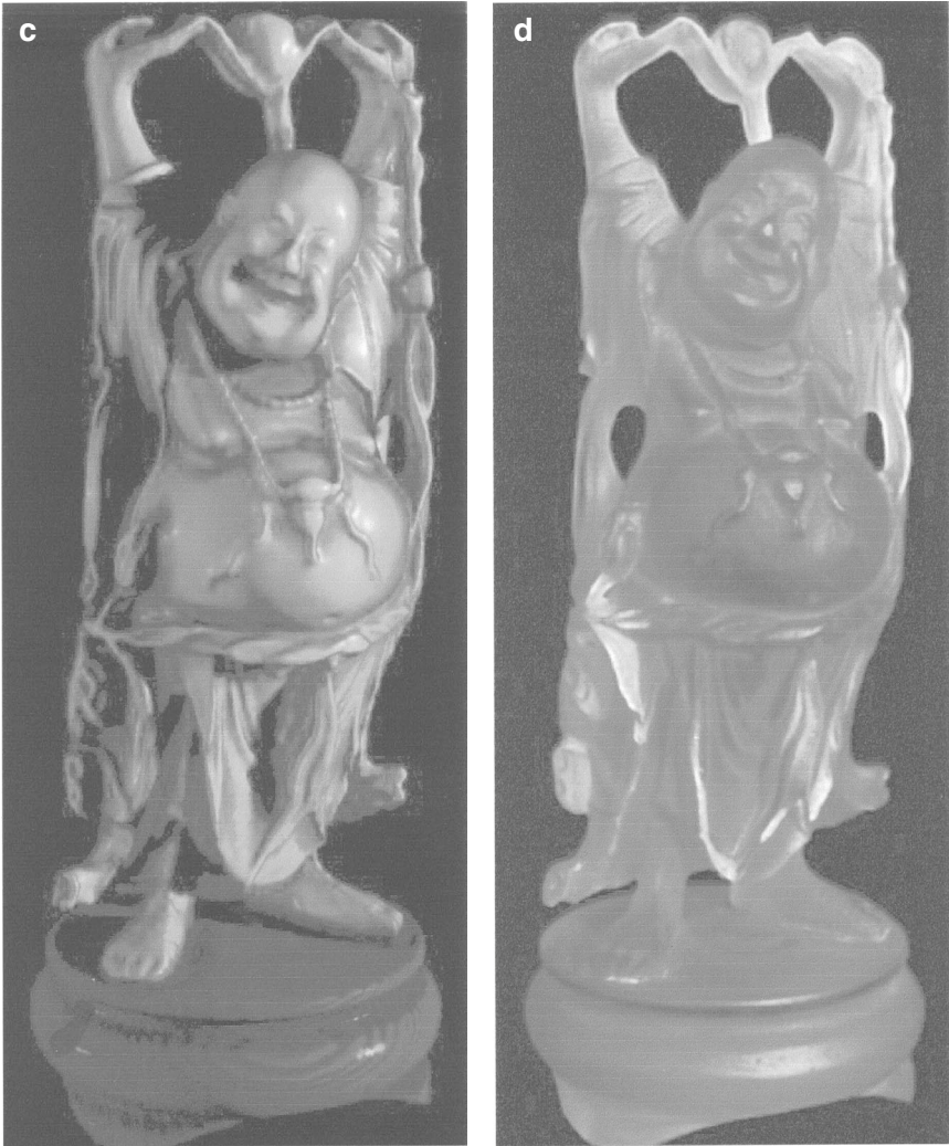
hours. (c) This is a colored (see website) and smooth-shaded rendering of this model. (d) Here is a photograph of a physical replica made from the computer model; the replica was manufactured by 3D Systems, Inc. which used a rapid prototyping technology called stereolithography. This process also takes several hours. Figures can be viewed in color at http://www-graphics.stanford.edu/projects/faxing/happy/ , figures (1), (3), (5), (6).
