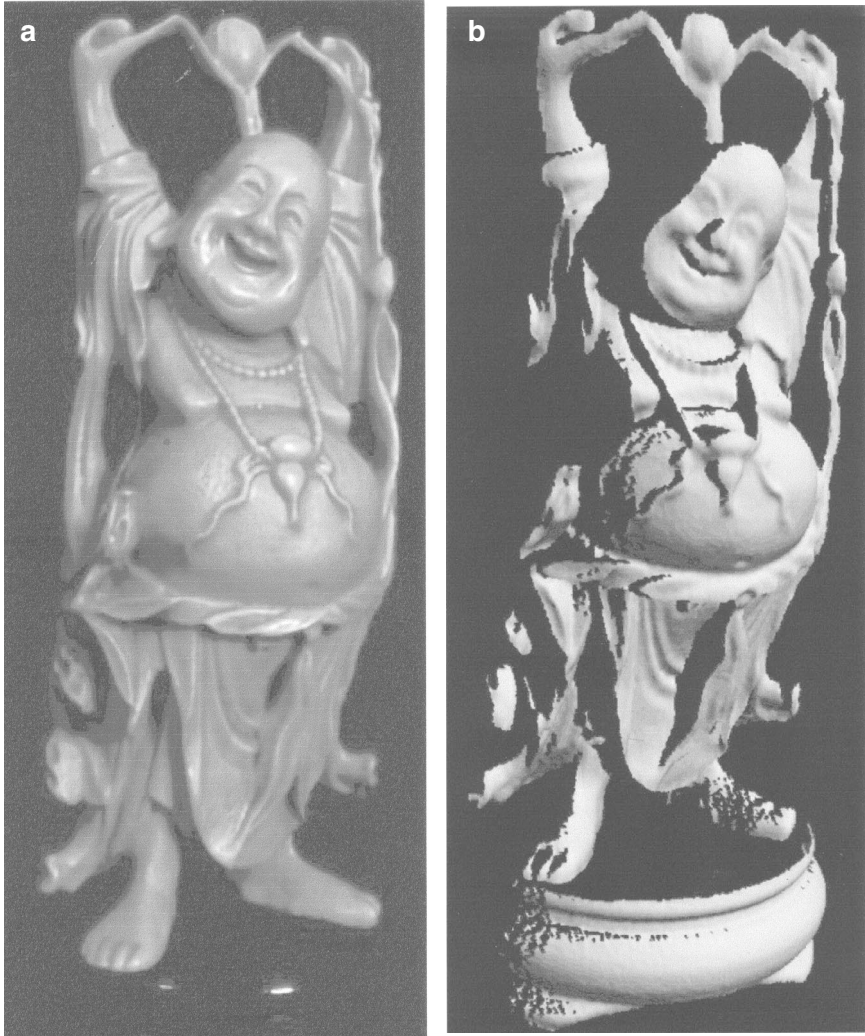
FIGURE 2 The Happy Buddha, from original to 3D fax. (a) This is a photograph of the plastic and rosewood statuette, which stands 20 cm tall. (b) Here we show a smooth-shaded computer rendering of one range image of the statuette. This figure illustrates the limited and fragmentary nature of the information available from a single range image. After digitizing and combining 58 such scans, we obtain a 2.6 million polygon mesh representing the entire statuette. The process takes several
