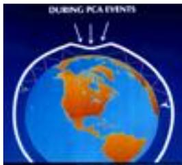
Illustration of the communications effects of ionospheric changes caused by solar proton events, known as Polar Cap Absorption (PCA) events (courtesy of M.A. Shea, Phillips Laboratory).
