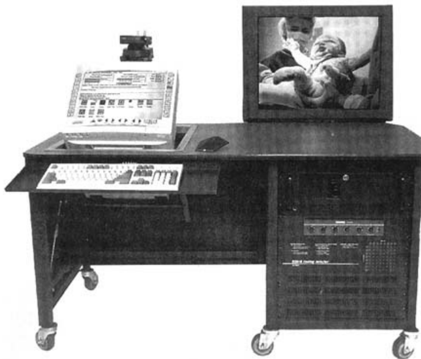
FIGURE 2.2 Telemedicine work station—an example as it might be configured with hardware and software for a consulting clinician to conduct live video conferencing, capture and transmit images and other data on a store-and-forward basis, share information from the patient record, and perform on-line medical literature searches. The unit includes a personal computer, robotic (pan-tilt-zoom) video camera (mounted above the computer monitor), large video display monitor, microphone, speakers, CODEC (an electronic COder/DECoder device), and software for a variety of purposes including control of some peripheral devices at the remote site. At the remote site, the installation would include a similar set up plus the peripheral devices (e.g., Doppler stethoscope, high-resolution digital still-image camera, full-motion video camera), document scanners, and other equipment appropriate for the patients to be evaluated. Photo used with permission of md/tv, inc., a subsidiary of Multimedia Medical Systems.
