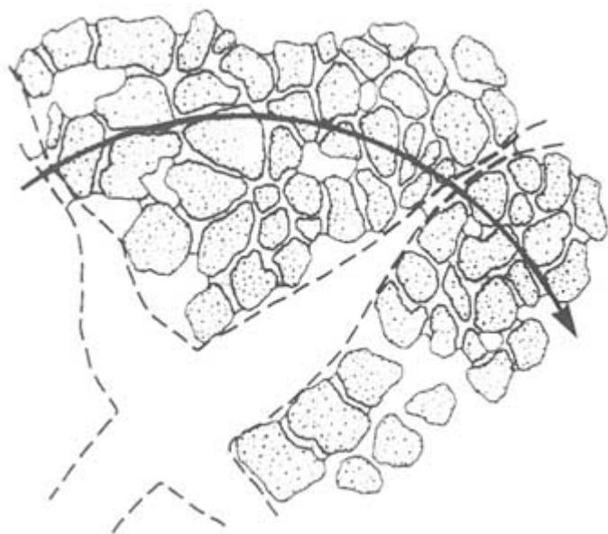
FIGURE 6.30 Conceptual model of flow in an unsaturated fractured rock. From Wang and Narasimhan (1985).
