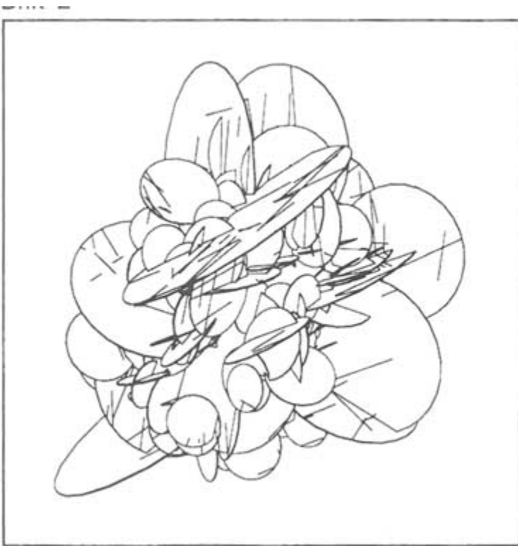
FIGURE 6.21 Example of a fracture network generated by using the parent-daughter process. From Billaux et al. (1989).
