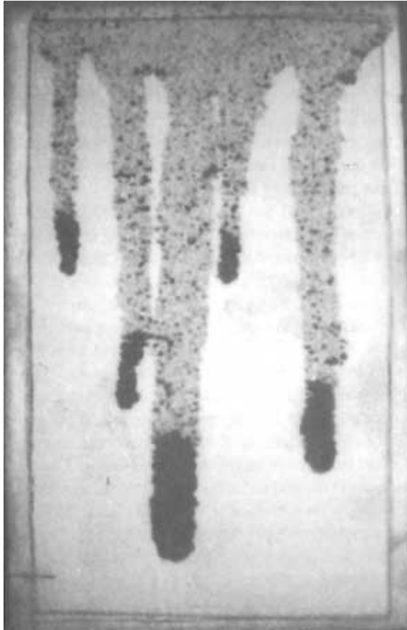
FIGURE 3.B2 Fingers originating from the stable front seen in figure 3.B1 . Partially saturated regions (mottled regions) are wetted near field capacity of the analog fracture. Courtesy of R. J. Glass.
