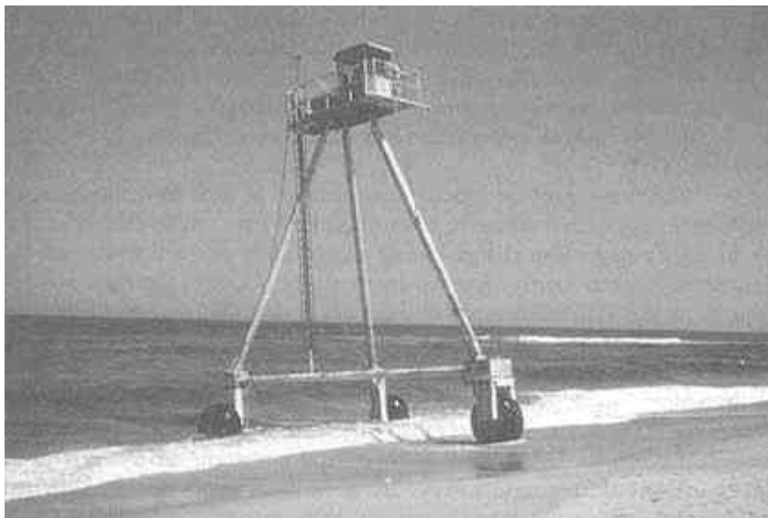
FIGURE G-2 Coastal Research Amphibious Buggy (CRAB), a sophisticated mobile survey station used to profile the seabed from the dune through the surf zone out to a water depth of 10 m.
