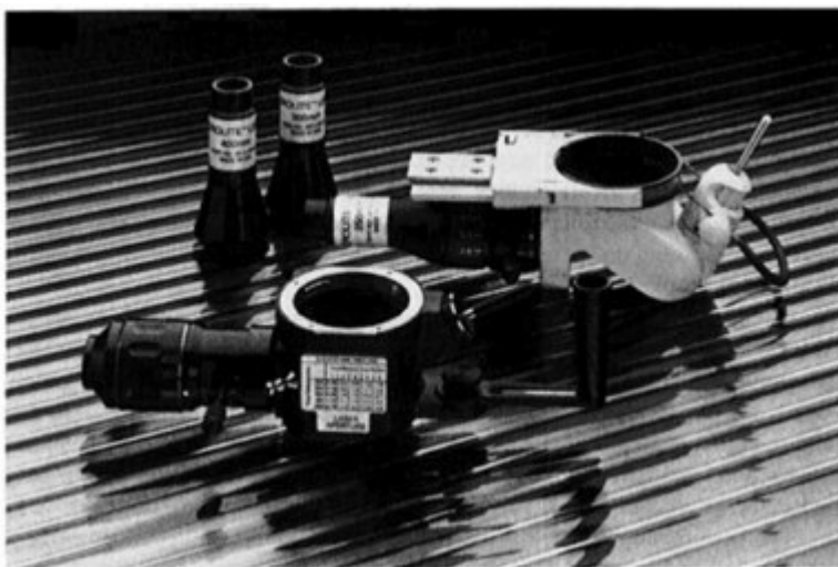
FIGURE 2.12 Micromanipulators used to deliver laser beams of very small diameter for precision work under the operating microscope. These micromanipulators accept the output of the laser and project a visible aiming beam, as well as the treatment beam, onto the surgical site in the field of view of the microscope. Controls on the micromanipulators allow the surgeon to move the beam within the microscope's field of view and to change the spot size. (Courtesy of Coherent, Inc., Palo Alto, Calif.)
