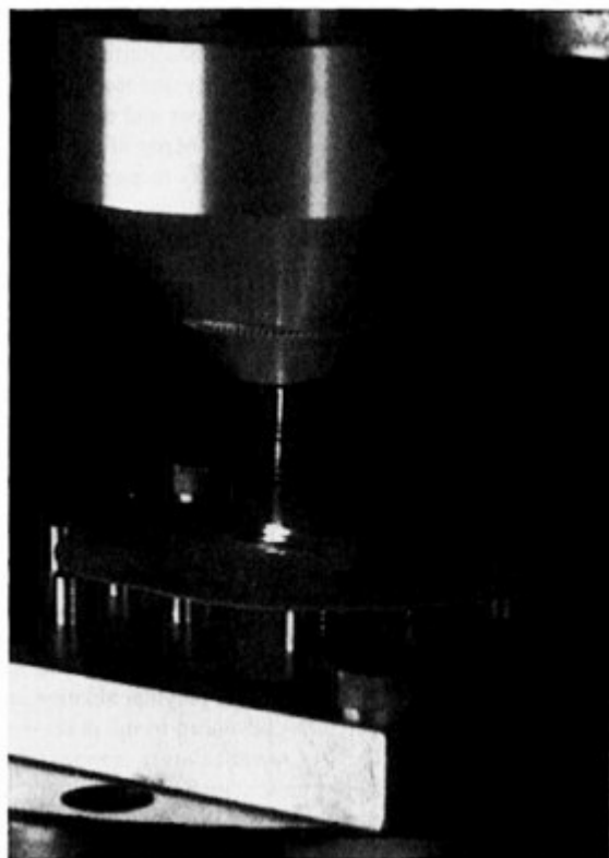
FIGURE 2.6 Nd:YAG laser beam mills precise three-dimensional undamaged patterns in a lithium tantalate crystal. Gears and other complex mechanical parts can be made with characteristic diameters of the order of a few times the diameter of a human hair. (Reprinted, by permission, from Eli Wiener-Avnear, "Lasers Cut Microscopic Paths with Major Potential," Laser Focus World 29 (July), 75-80, 1993. Copyright © 1993 by PennWell Publishing Co.)
