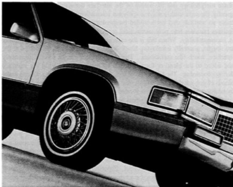
FIGURE 3.5 High-performance alloys are now used extensively in the demanding exterior body applications of automobiles. For example, front fenders are molded from a PPO-nylon alloy that can withstand paint oven temperatures of 400°F and above. They are chosen for their class-A surface, dimensional stability, impact strength, and corrosion and chemical resistance. The side claddings on these vehicles are molded of a resin that is a polyester-polycarbonate alloy, chosen for its cold temperature impact strength, chemical resistance, and quality surface. For the front and rear bumper fascias, a copolyester elastomer is used, characterized by its cold temperature ductility, class-A surface, chemical resistance, and on-line paintability at temperatures exceeding 280°F. More than 60 pounds of engineering thermoplastics can be found on many of the vehicles. SOURCE: Photograph courtesy of GE Plastics, Southfield, Michigan.
