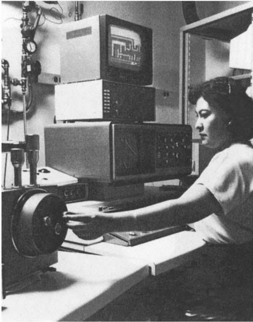
Maria Isabel Soto uses a scanning electron microscope to find defects in an electrical circuit.
