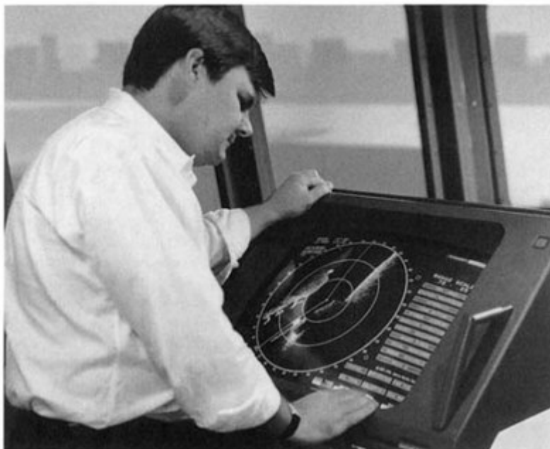
ARPA radar in use "aboard" a full-mission ship bridge simulator. (STAR Center Dania, Florida, American Maritime Officers)
