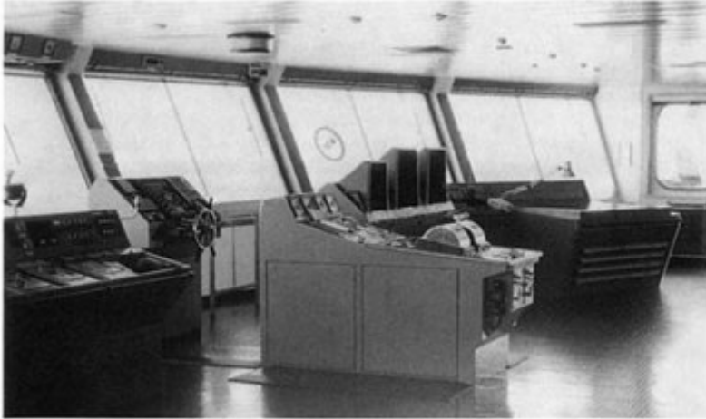
Integrated bridge system aboard the Regal Princess . (Sperry Marine, Inc.)
