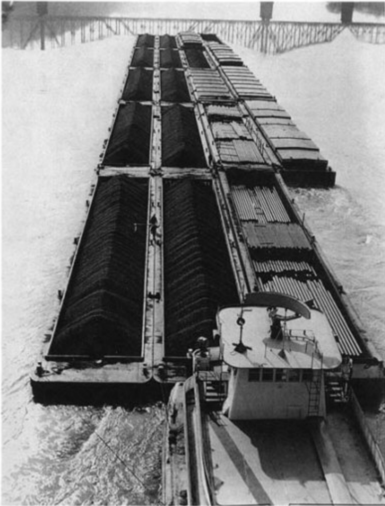
River tug and tow in push-tow configuration. The specific skills required to maneuver river tows differ from those required to maneuver ships, because of significant differences in maneuvering characteristics and differing steering equipment employed aboard river towboats. ( American Waterways Operators )
