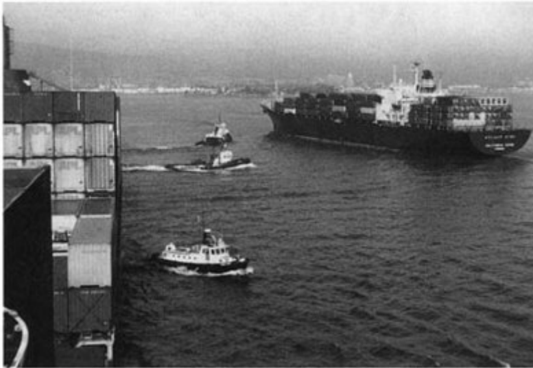
Pilot boarding area just seaward of Los Angeles Harbor. The pilot boat is shifting the marine pilot from the outbound U.S.-flag container ship to an inbound foreign-flag container ship. The assist tugs are shifting from the outbound to the inbound ship to await the pilot's instructions once the pilot has boarded from the pilot boat.(William A. Creelwman)
