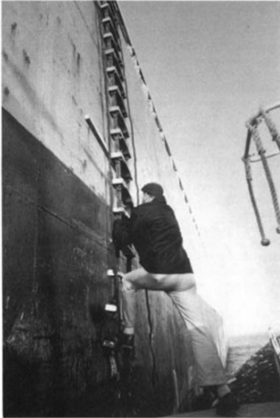
Bar pilot stepping from a pilot boat to a pilot ladder while boarding a ship off San Francisco in good weather. (Joseph A. Zygaj, San Francisco Bar Pilots )
