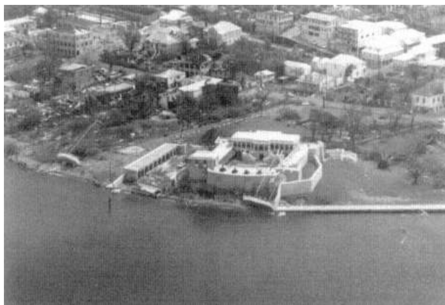
Figure 6-7 St. Croix, northern shore, west of Christiansted. Reduced penetration of storm surge owing to steep terrain (see also Figures 6-5 and 6-6 ). Courtesy: Richard Marshall, 1989.
