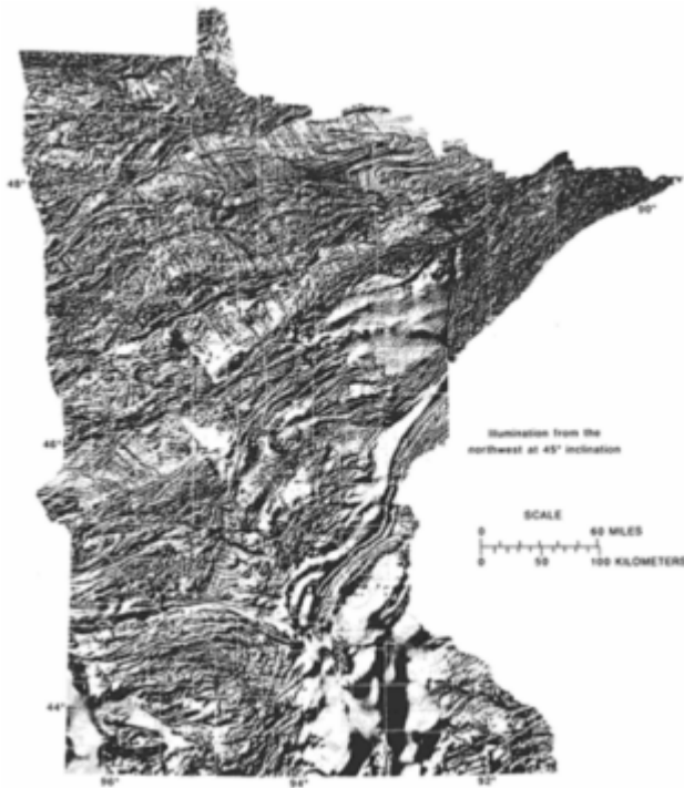
Figure 3-1 Shaded relief image of high-resolution aeromagnetic data from Minnesota (courtesy of the Minnesota Geological Survey). Most of the data used to produce this image were acquired under the supervision of the Minnesota Geological Survey; additional data were contributed by the U.S. Geological Survey, USX Corporation, and the Geological Survey of Canada.
