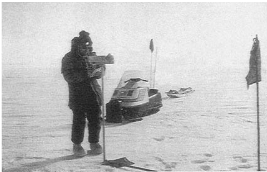
FIGURE 4.4 A researcher has traveled by snow mobile to a remote site in order to operate an electronic distance-measuring device on the ice sheet. Surveys of networks of such markers provide glaciologists data on the flowrates and deformation rates of the ice sheet. (Courtesy of R. Bindshadler, NASA Goddard Space Flight Center).
