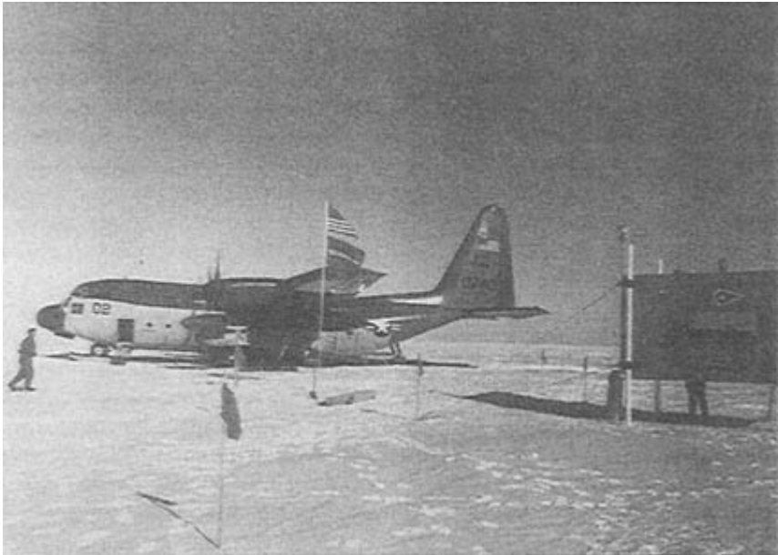
FIGURE 2.1 The first Automatic Geophysical Observatory (AGO) set up for unmanned operations at a remote site in Antarctica 500 km from the South Pole. The ski-equipped Hercules aircraft is positioned to deliver the year's supply of propane that fuels the AGO's 60 watt thermoelectric generator. Heat from the generator is used to maintain the shelter at a constant room temperature while the experiment electronics pass nearly 3 gigabytes of science data to the AGO's recorders. Six instruments supplied by one Japanese and five U.S. institutions are included in the instrument complement for studies of upper atmosphere physics. Also included is a set of meteorology instruments. (Courtesy of J.H. Doolittle, Lockheed Palo Alto Research & Development Laboratory. Acknowledgement: NSF/OPP contract DPP 88-14294).
