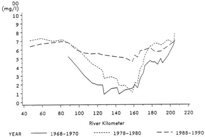
FIGURE 1.4a Historic summer dissolved oxygen profiles for the Delaware Estuary. (Source: Marino et al. 1991. Reprinted, by permission, from Najarian Associates, 1991.).
