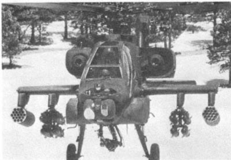
Figure 1 AH-64 Apache attack helicopter. NOTE: The AH-64 Apache attack helicopter represents the utmost in modern air weaponry. The two-man airframe system is designed to fly in literally any weather conditions.
