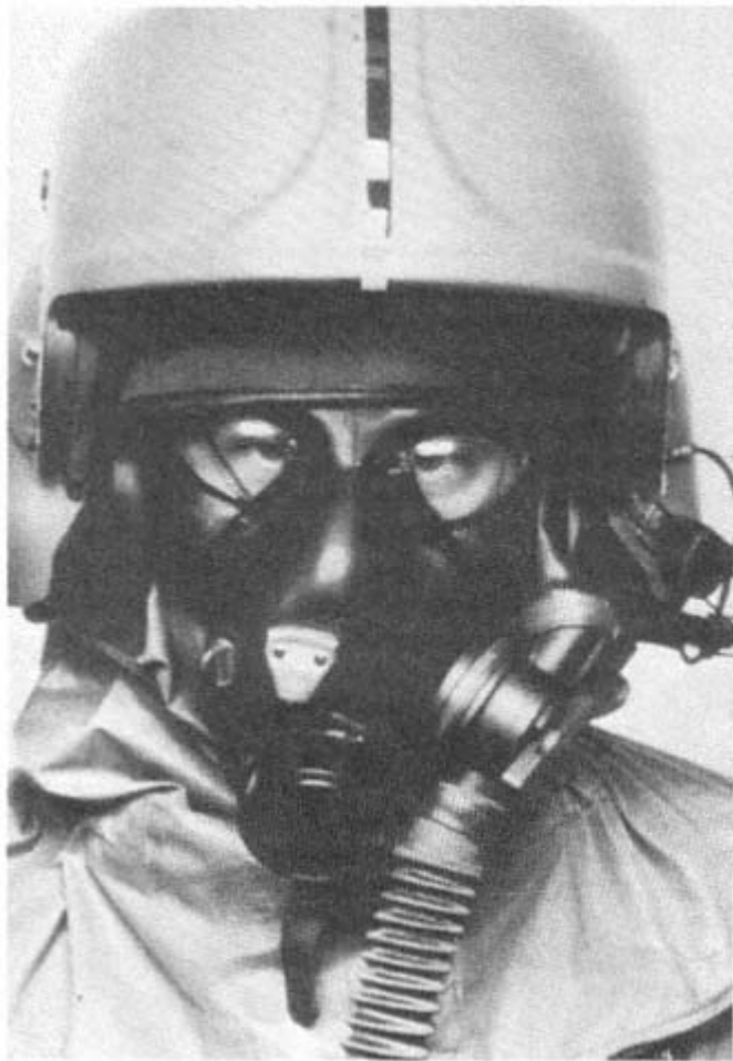
Figure 3 U.S. Army M-48 protective mask. NOTE: The M-48 protective mask was designed specifically for the Apache system, since the preexisting M-24 protective mask was totally incompatible with HDU positioning.
