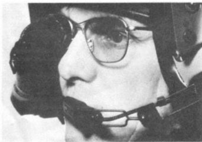
Figure 2 U.S. Army helmet display unit. NOTE: The HDU is positioned over the right eye; spectacle-wearing aviators have had some difficulty in obtaining proper positioning for optimal utilization.
