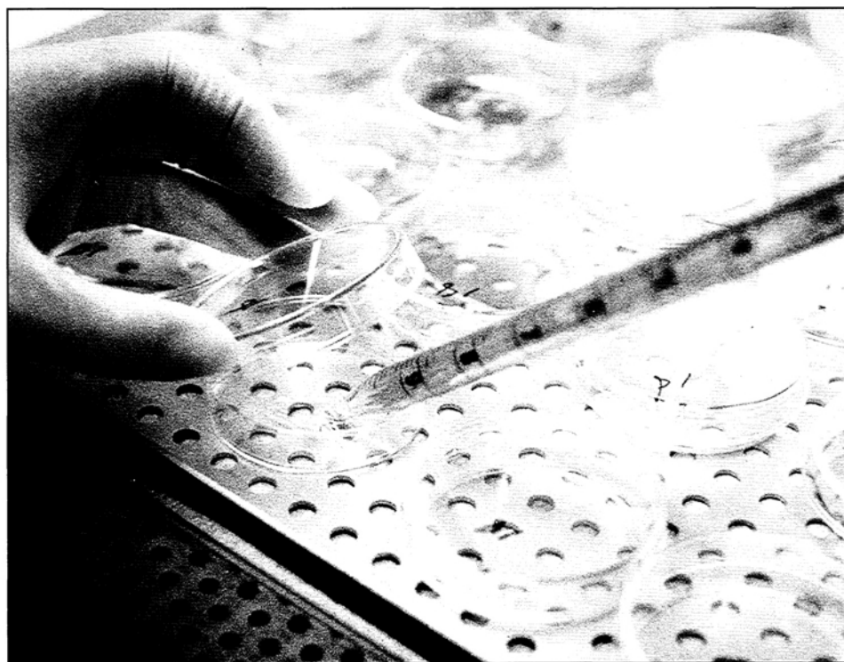
A technician pipets into a culture dish used to test the effects of chemicals on cultured hamster embryo cells.
