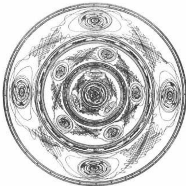
Figure 9. Fractal structure near a periodic orbit: islands signal resonances of various orders, while tangles represent regions of chaos.
