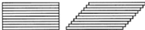
Figure 10. The same set of rods that forms a rectangle can also form a parallelogram of the same dimensions. Hence the areas of the rectangle and the parallelogram must be the same.
