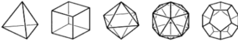
Figure 1. The five regular polyhedra. Each is composed of a single type of regular polygon, with the same number of polygons meeting at each corner. The tetrahedron, octahedron, and icosahedron are made of triangles, the cube is made of squares, and the dodecahedron is made of pentagons.
