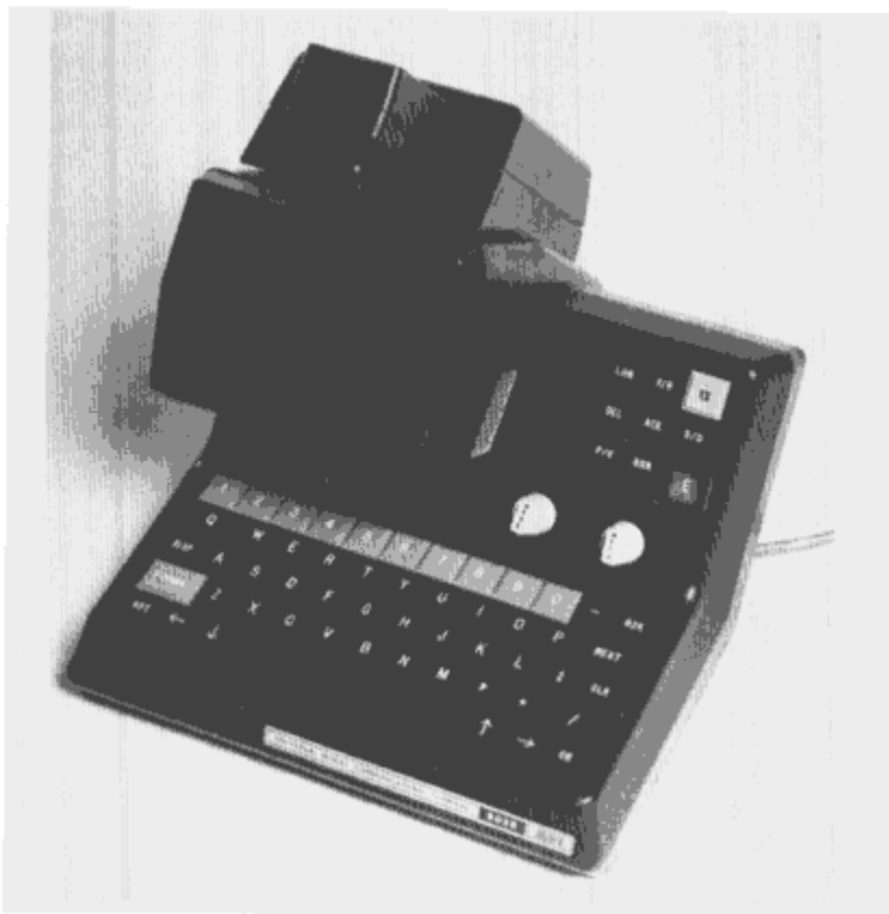
Figure 3 DADS Mobile terminal. The "shoe" for the scanner, shown in this photograph, was added after DADS implementation.
