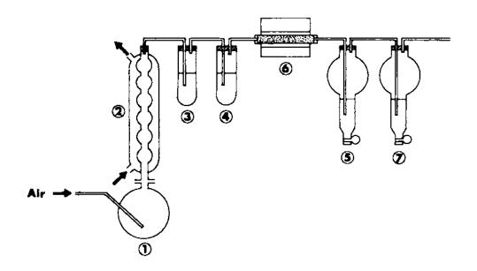
Figure 2 Apparatus for carbon separation in sulfuric baths. 1 - dissolution flask, 2 - refrigerant, 3 - HF - HNO3 - H2O (2 - 2 - 1) in volume) absorber  $(40 \text{ cm}^3)$ , 4 - 9M HNO3 absorber  $(40 \text{ cm}^3)$ , 5 -copper oxide on porous alumina in a furnace at  $800^{\circ}\text{C}$ , 6, 7 - 12M KOH absorbers  $(10 \text{ cm}^3)$  each).
