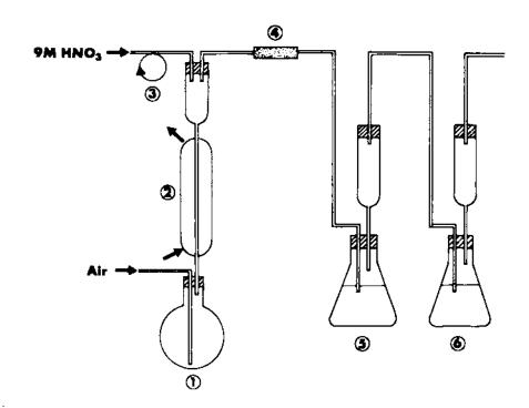
Figure 1 Apparatus for the separation of carbon. 1 - flask for the dissolution of the solid residue of the alkaline bath, 2 - refrigerant, 3 - peristaltic pump, 4 - quartz-wool filter, 5,6 - 12 M KOH absorbers.
