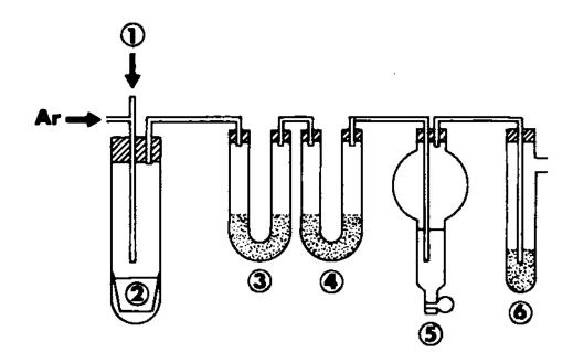
Figure 4 Apparatus for the radiochemical separation of nitrogen and carbon from silicon. 1 - sample introduction, 2 - KOH in nickel crucible at 500°C, 3 - granulated CuO at 900°C, 4 - CuO on porous alumina at 900°C, 5 - 12M KOH, 6 - titanium sponge at 900°C.
