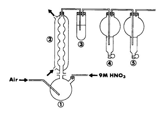
Figure 3 Apparatus for carbon separation after fusion in alkaline baths. 1 - dissolution flask, 2 - refrigerant, 3 - 9M HNO3, absorber (40 cm $^3$ ), 4,5 - 12M KOH absorbers (10 cm $^3$  each).
