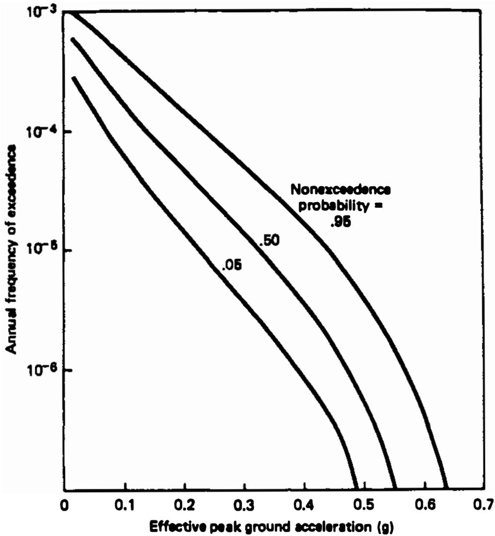
FIGURE 3.3 Seismic hazard curves for a hypothetical site (Office of Nuclear Regulatory Research, 1981).
