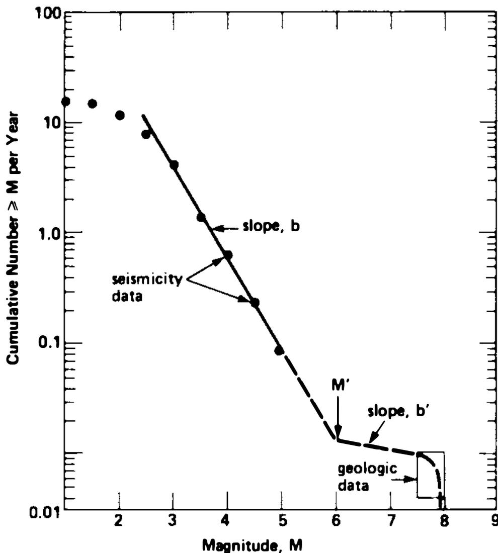
FIGURE 3.4 Diagrammatic cumulative frequency-magnitude recurrence relationship for an individual fault or fault segment. Above magnitude  $M'$  a low  $b$  value ( $b'$ ) is required to reconcile the small-magnitude recurrence with geologic recurrence, which is represented by the box. (From Schwartz and Coppersmith, 1984.)
