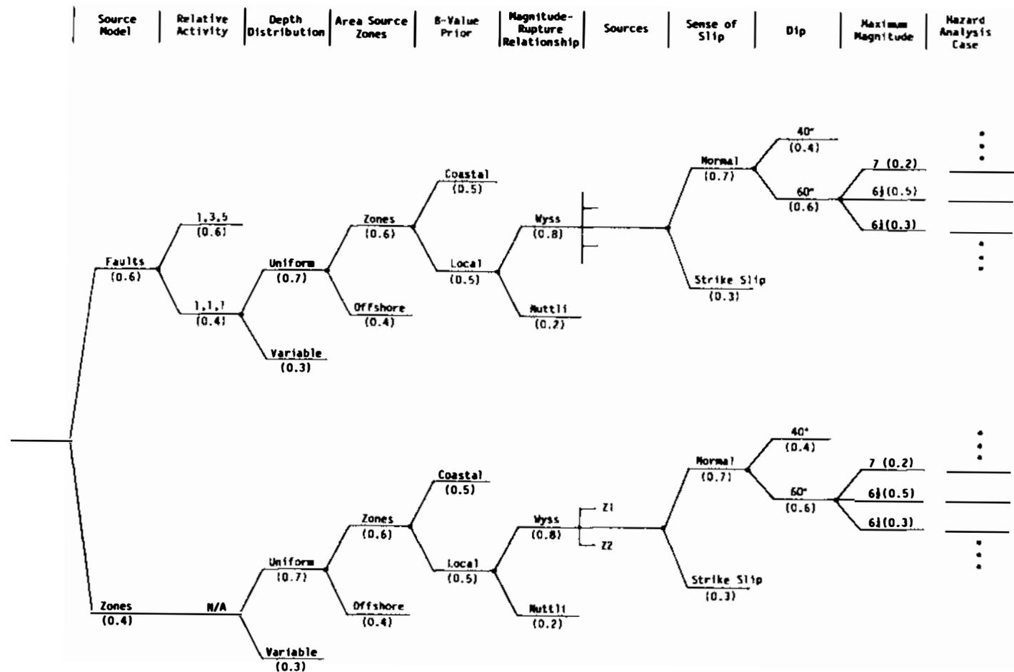
FIGURE 3.5 Example logic tree for seismic sources in the North Sea (After Coppersmith and Youngs, 1986).
