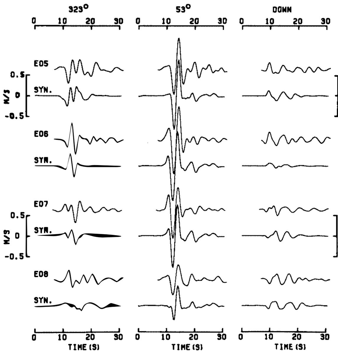
FIGURE 6.3 Comparison of observed and computed ground velocity at four sites in the October 1979 Imperial Valley earthquake (Archuleta, 1984).
