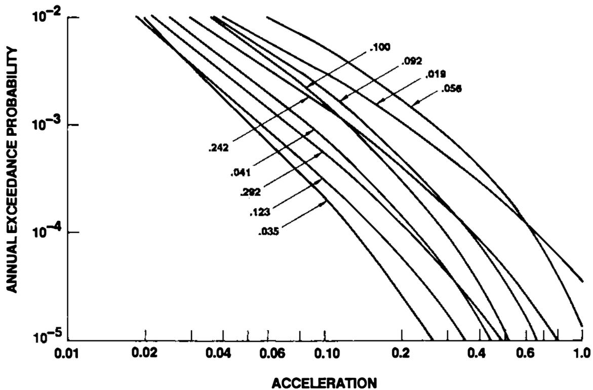
FIGURE 3.2 Typical seismic hazard analysis results for particular site. Number for each curve is weight assigned to analysis. Seabrook Station Probabilistic Safety Assessment. Reprinted by permission from Public Service Co. of New Hampshire (1983).
