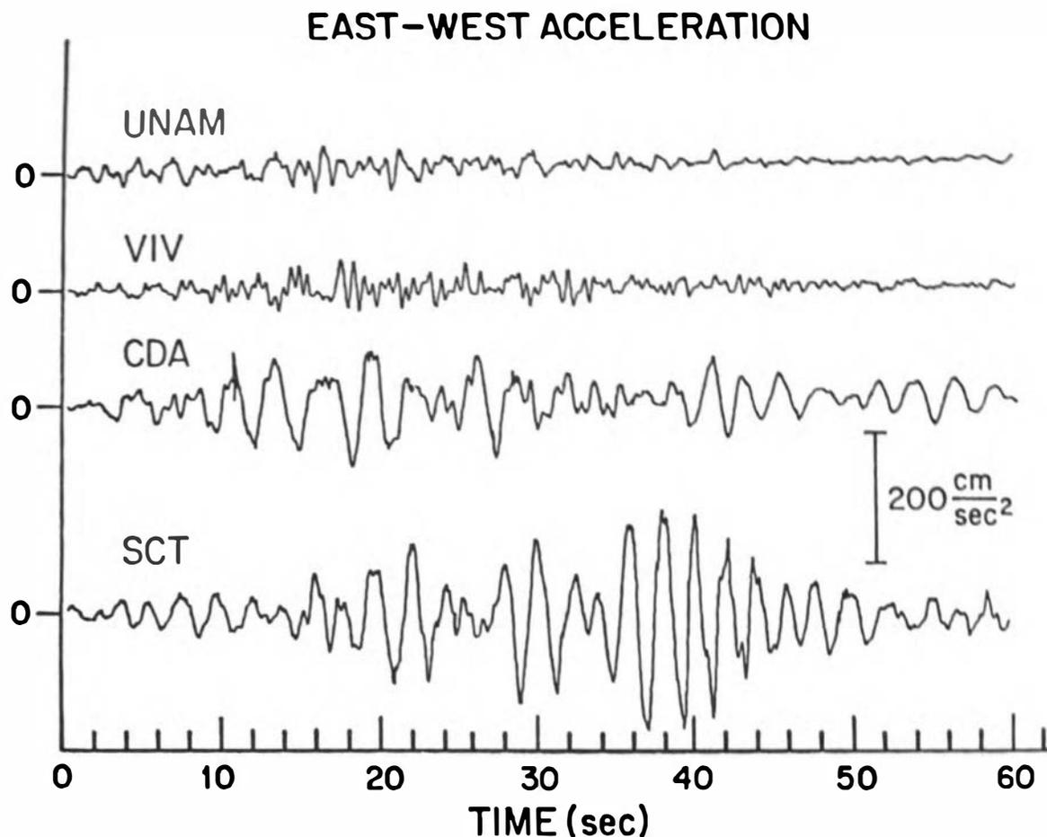
**FIGURE 6.4** Most significant one-minute segments of the east-west acceleration recorded on the free-field accelerographs in Mexico City. No time correlation exists between these traces (Anderson et al., 1986). The UNAM record was taken on a recent basalt flow; the VIV was recorded on firm alluvial and lake deposits; the CDA and SCT records were recorded on deep, soft, lake bed deposits. These four stations are separated by 10 km or less, and are 300 km from the earthquake source.
