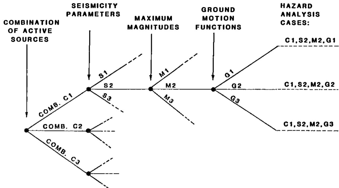
FIGURE 2.7 Example of logic tree format used to represent uncertainty in hazard analysis input. Each branch has an assigned weight and the sum of weights on branches attached to any node is unity (McGuire, 1986). Reprinted by permission from R. K. McGuire.
