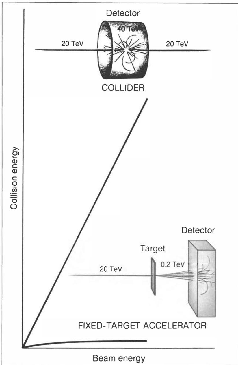
**FIGURE 2** The advantage of a collider.
