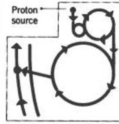
Injection system loading protons into counterclockwise beam pipe of main ring
