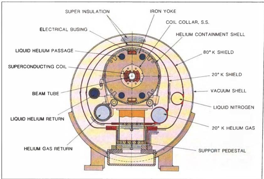
**FIGURE 4** Detail of magnet assembly.
