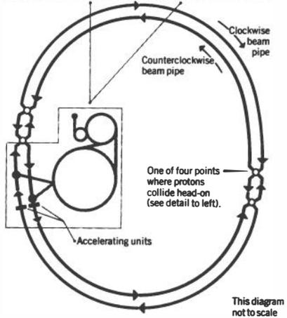
**Main ring sustaining dual proton beams**
